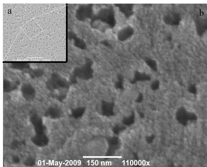
**Fig. S12** FE-SEM images of the hierarchically macro-/meso-/micro-porous carbon material after washing away the CaO particles of the composites, which are obtained from the mesoporous composite CaO/C-4-700 after 10 cycles of CO<sub>2</sub> absorption and regeneration.
