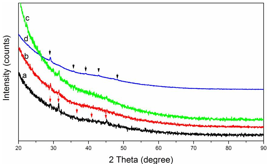
**Fig. S5** Wide-angle XRD patterns of the mesoporous composites obtained by pyrolyzing the as-made CaO/C-3 composite at a) 350, b) 400, c) 500 and d) 600 °C under Ar. The marked red arrows are supposed to ascribed to Ca(NO<sub>2</sub>)<sub>2</sub> (JCPDS 280-232) while the black ones to CaCO<sub>3</sub> (JCPDS 862343).
