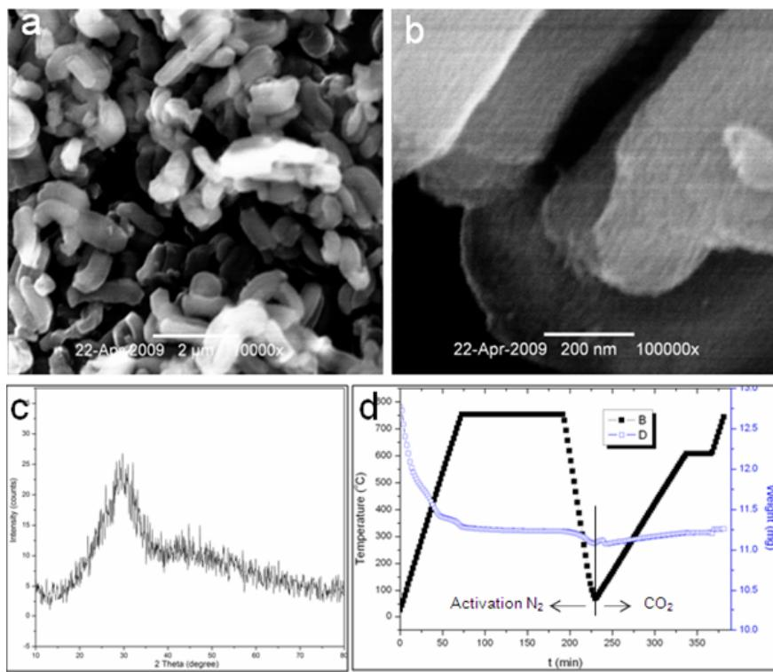
**Fig. S13** FE-SEM images (a, b), wide-angle XRD pattern (c) and the temperature-dependent CO<sub>2</sub> sorption behavior (d) of the mesoporous silica SBA-15 loaded with ~ 35 wt % of CaO.
