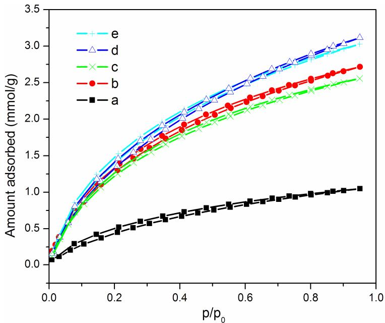
**Fig. S7** CO<sub>2</sub> adsorption isotherms at 25 °C of the ordered mesoporous CaO/C composites obtained by heating the as-made CaO/C-3 sample under Ar at a temperature of a) 350, b) 500, c) 600, d) 700 and e) 900 °C, respectively.
