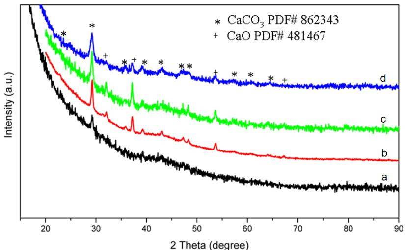
**Fig. S6** Wide-angle XRD patterns of the mesoporous composites CaO/C-x-700 obtained by pyrolysis at 700 °C under a gas atmosphere of 2.4 % O<sub>2</sub> in N<sub>2</sub>.
