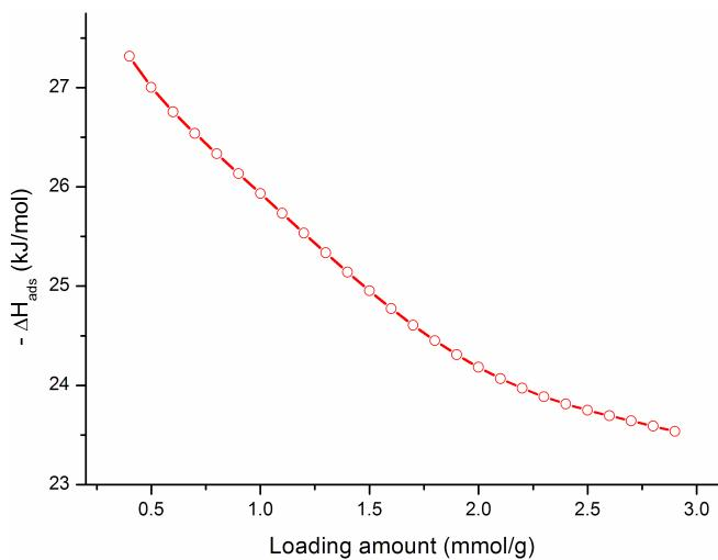
**Fig. S8** Dependence of the isosteric heats of adsorption as function with loadings for adsorption CO<sub>2</sub> on the ordered mesoporous composites CaO/C-3-900 with a CaO content of 15.8 wt %.
