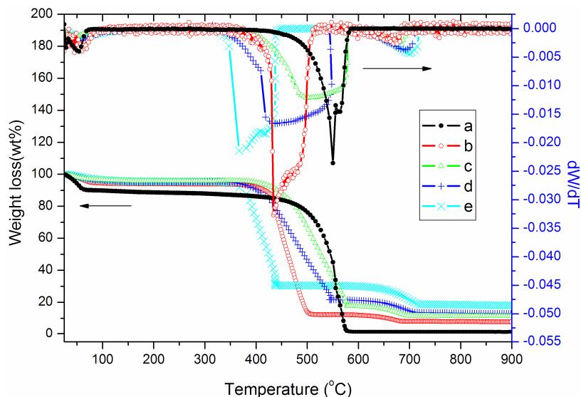
**Fig. S3** TG and DTG curves (conducted under O<sub>2</sub>) of a) the calcium-free mesoporous carbon sample and the mesoporous calcium oxide/carbon composites with the CaO content of b) 8.0, c) 11.5, d) 13.5 and e) 18.5 wt %. The combustion temperature lowers down considerably from ~ 580 °C for the pure carbon sample to ~ 420 °C for the composites with 18.5 wt % of CaO. During the combustion, calcium carbonate is formed first and then fully decomposed at ~ 680 °C.
