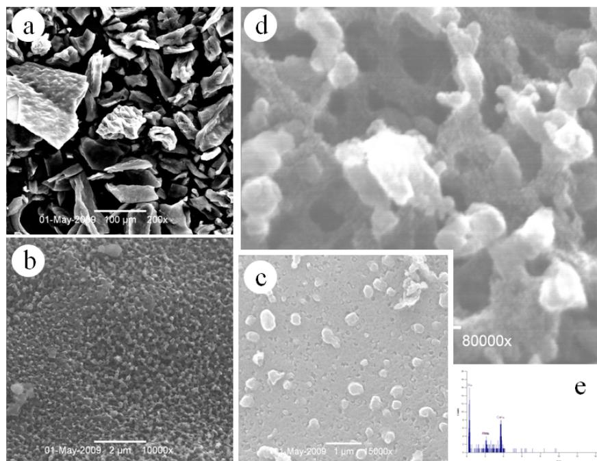
**Fig. S11** FE-SEM images (a-d) and EDX spectrum (e) of the residues obtained from the mesoporous composites CaO/C-4-700 after ten cycles of CO<sub>2</sub> absorption and regeneration.
