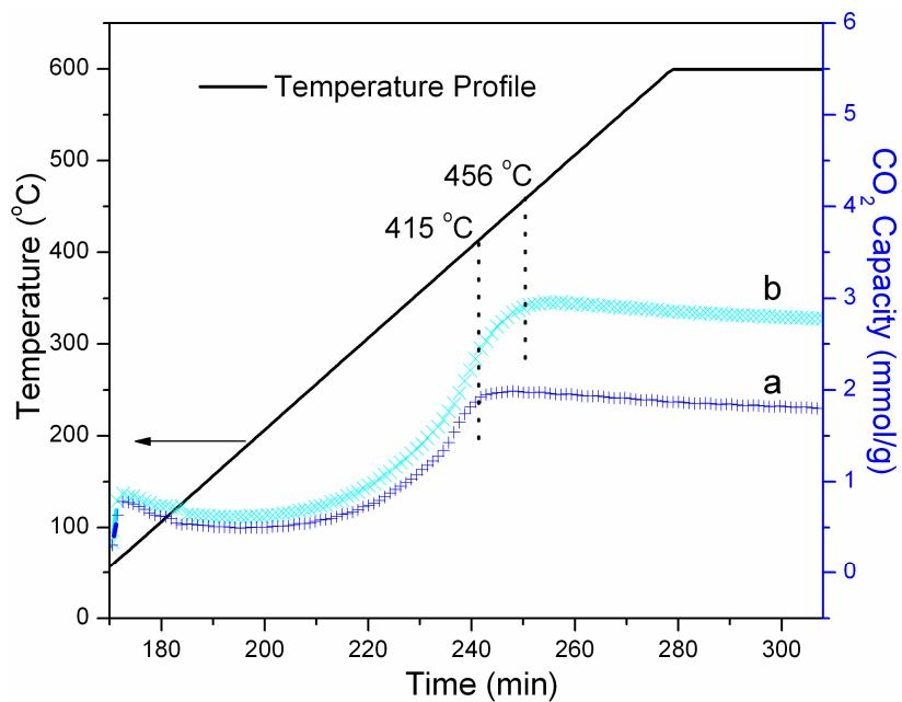
**Fig. S9** CO<sub>2</sub> sorption amount as a function of temperature of the mesoporous composites obtained at 700 °C with a calcium content of 13.5 and 18.5 wt %, respectively.
