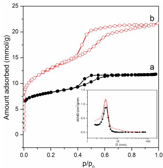
**Fig. S4** N<sub>2</sub> sorption isotherms of a) the mesoporous CaO/C composites obtained at 700 °C with CaO content of ~ 14 wt % and b) the corresponding mesoporous carbon material after washing away the calcium component by 2 M HCl solution at 50 °C overnight. High surface area and pore volumes are obtained after the treatment, indicating a good *in-situ* activation effect of the carbon support by calcium oxide at high temperatures.
