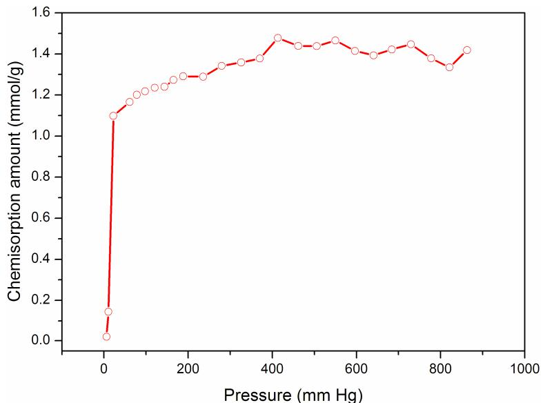
**Fig. S10** Chemisorption isotherm of CO<sub>2</sub> at 450 °C of the mesoporous composites CaO/C-4-700 with a CaO content of 18.5 wt %. The capacity is calculated to be ~ 1.5 mmol/g, which is lower than the value obtained by thermogravimetric analysis. The reason is that the activation temperature is only 450 °C limited by the analyzer. In this case, part of the calcium is in the form of carbonate before the analysis.
