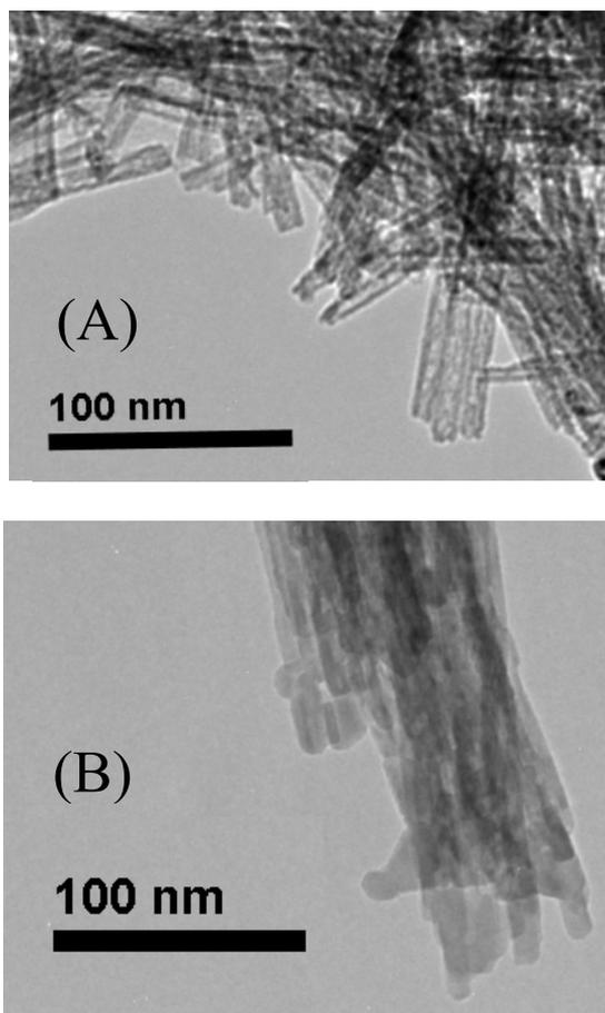
Fig. S2. TEM image of titania nanotubes (A) and anatase nanorods (B)
