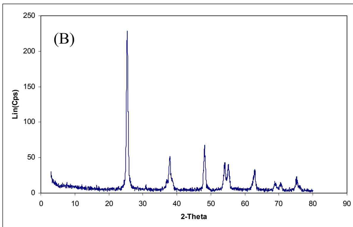
Figure S1. XRD spectrum of titania nanotubes (A) and anatase nanorods (B)
