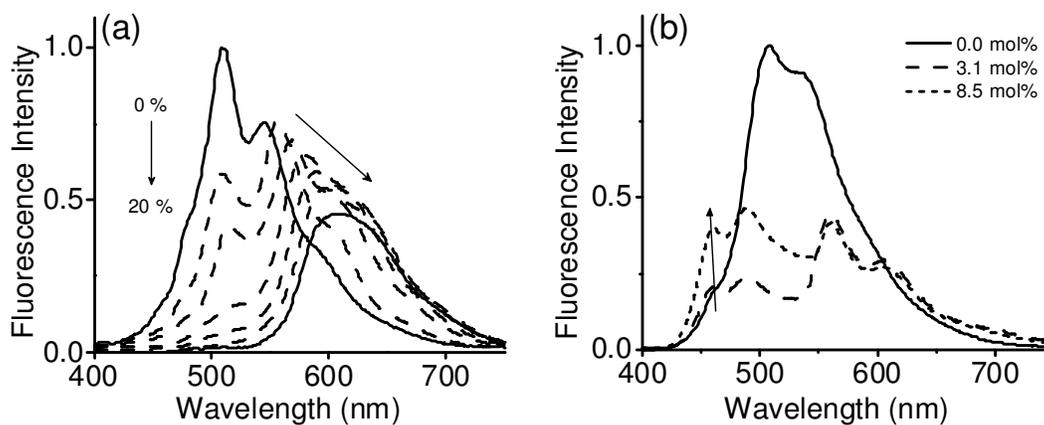
**Fig. S6** Fluorescence spectral changes of (a) **OPV1** and (b) **OPV3** in presence various amounts of **OPV5** in *n*-decane at room temperature (conc. of donor =  $3 \times 10^{-4}$  M,  $l = 1$  mm,  $\lambda_{\text{ex}} = 380$  nm).
