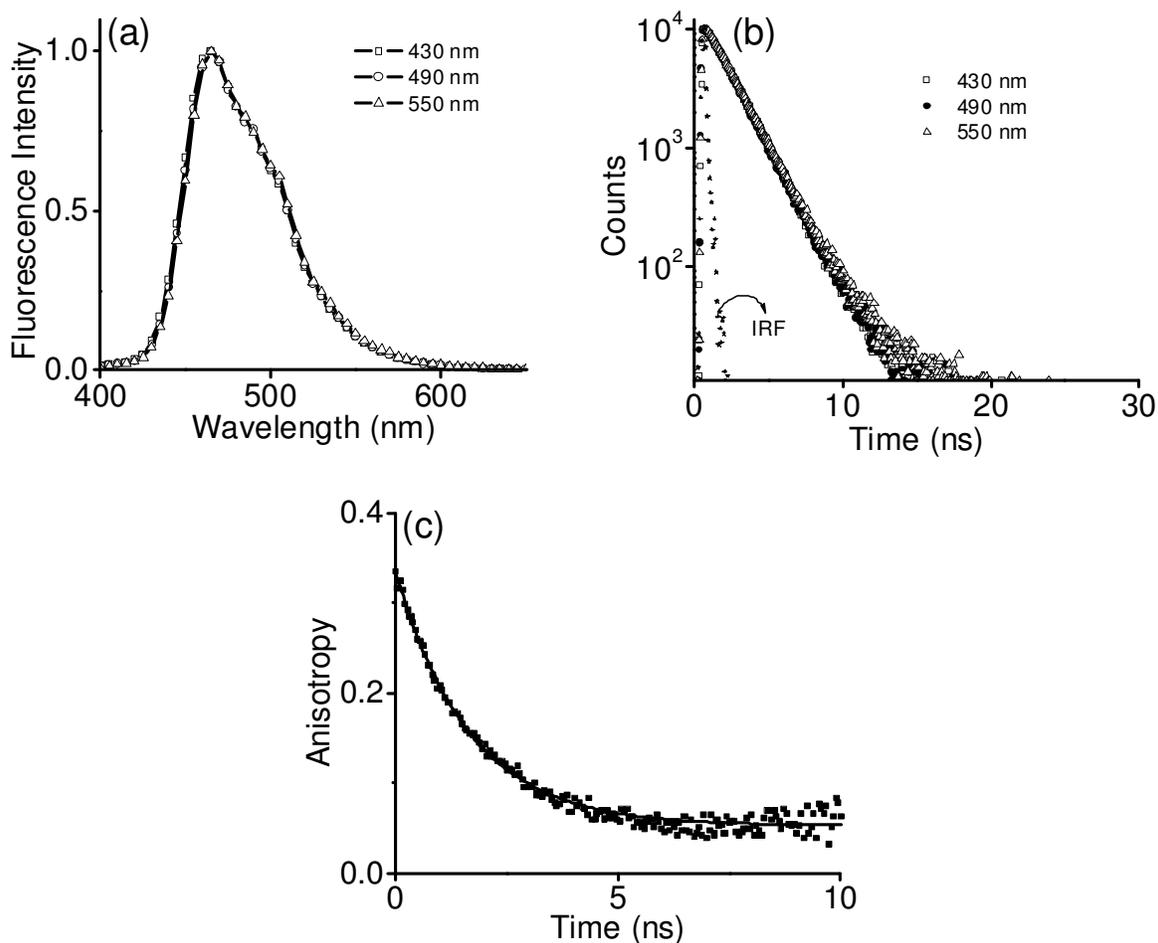
**Fig. S4** (a) Time-resolved emission spectra, (b) wavelength dependent fluorescence decay and (c) fluorescence anisotropy decay of **OPV1** in chloroform at room temperature.  $c = 3 \times 10^{-4}$  M,  $l = 1$  mm,  $\lambda_{\text{ex}} = 375$  nm.
