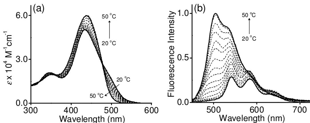
**Fig. S1** Temperature dependent (a) absorption and (b) emission spectral changes of **OPV2** in *n*-decane.  $c = 3 \times 10^{-4} \text{ M}$ ,  $l = 1 \text{ mm}$ ,  $\lambda_{\text{ex}} = 420 \text{ nm}$ .
