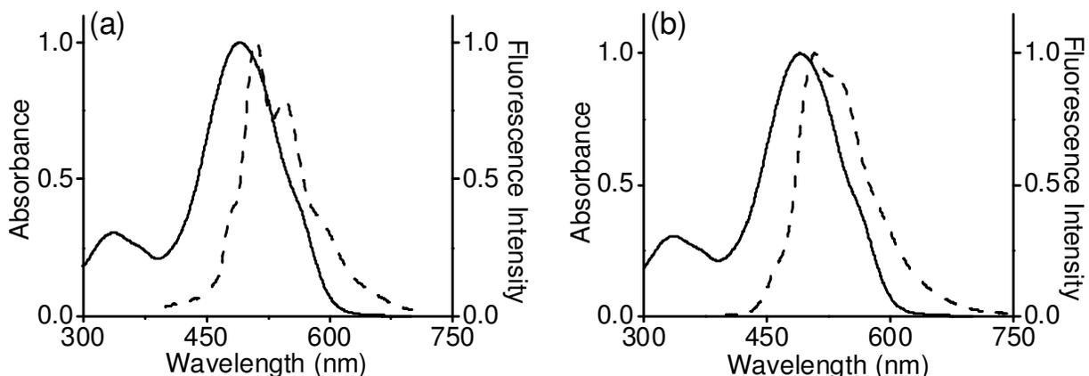
**Fig. S5** Spectral overlap of the absorption (—) of **OPV5** and emission (---) of (a) **OPV1** and (b) **OPV3** in *n*-decane at room temperature (conc. of donor =  $3 \times 10^{-4}$  M, conc. of acceptor =  $9.3 \times 10^{-6}$  M,  $l = 1$  mm,  $\lambda_{\text{ex}} = 380$  nm).
