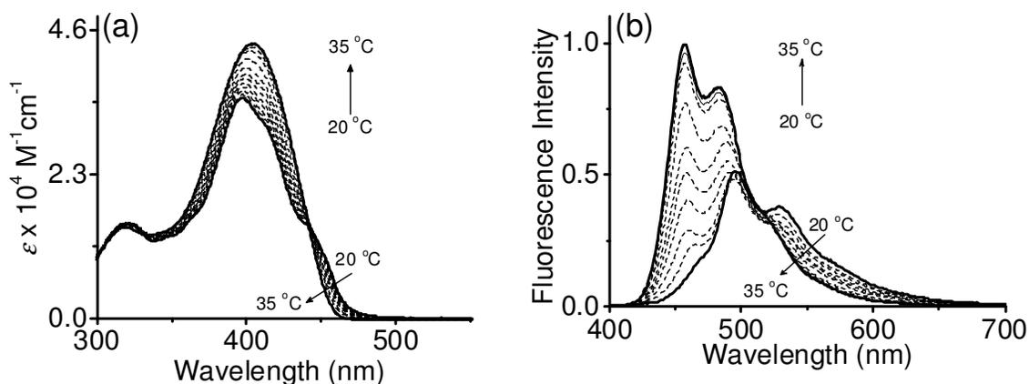
**Fig. S3** Temperature dependent (a) absorption and (b) emission spectral changes of **OPV4** in *n*-decane at room temperature.  $c = 3 \times 10^{-4}$  M,  $l = 1$  mm,  $\lambda_{\text{ex}} = 380$  nm.
