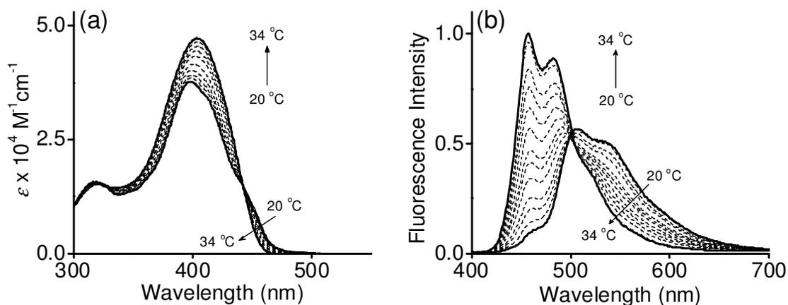
**Fig. S2** Temperature dependent (a) absorption and (b) emission spectral changes of **OPV3** in *n*-decane.  $c = 3 \times 10^{-4} \text{ M}$ ,  $l = 1 \text{ mm}$ ,  $\lambda_{\text{ex}} = 380 \text{ nm}$ .
