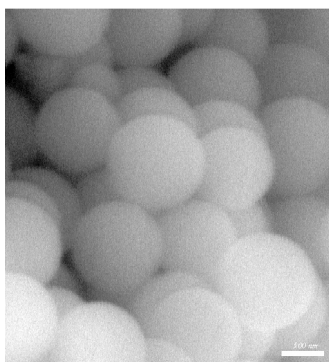
Figure ESI-3. ESEM Images of 1 \mu\text{m} monodisperse colloidal silica particles synthesized by following Table 1 parameters (Scale bar: 500nm).
