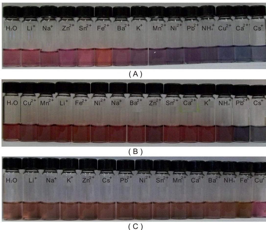
**Figure S1.** Photos showing the color changes for the methylthio-*t*-BCA molecules capped gold nanoparticles in response to the addition of different ions ( $M^{(n+)}Cl_n^-$ ). (A) Au@1; (B) Au@2; (C) Au@3.
