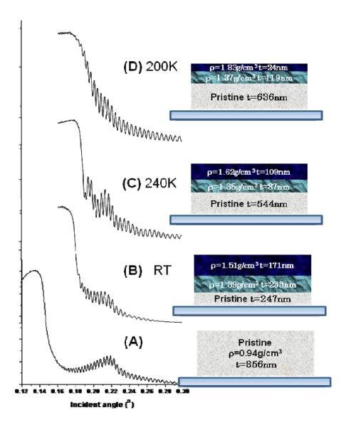
**Figure S1** XRR data and schematics of the film shrinkage (not-to-scale) and densities before (A) and after plasma exposure at room temperature (RT, 296K) (B), 240K (C) and 200K (D).
