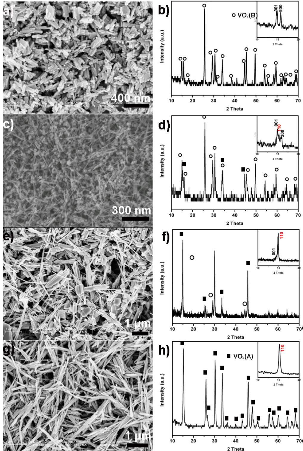
**Figure S2.** VO<sub>2</sub> samples treated at 200 °C for different hydrothermal periods. The left part shows the SEM images for the intermediate products for the morphology evolution from VO<sub>2</sub> (B) samples (a), VO<sub>2</sub> (B)+VO<sub>2</sub>(A) (c, e), and VO<sub>2</sub>(A) (g) during the formation process of VO<sub>2</sub>. The right part shows the corresponding XRD patterns for the intermediate products reacting after 10 h (b), 30 h (d), 36 h (f), and 40 h (h).
