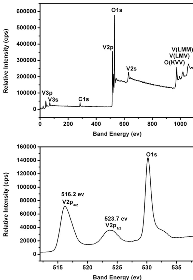
**Figure S3.** XPS spectra of VO<sub>2</sub> (A) nanobelts: (a) survey spectrum and (b) core-level spectra of V 2p and O 1s.
