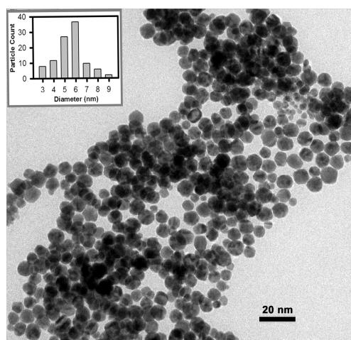
**Figure S2:** Low-Resolution TEM (LRTEM) image of bare ZnO NPs (inset shows particle size distribution of ZnO NPs).
