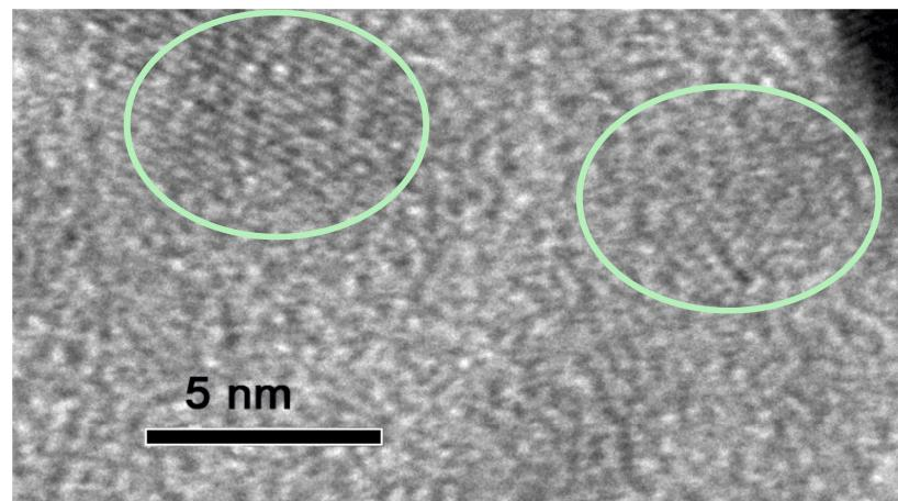
**Figure S1:** High-resolution TEM (HRTEM) image of bare ZnO NPs.
