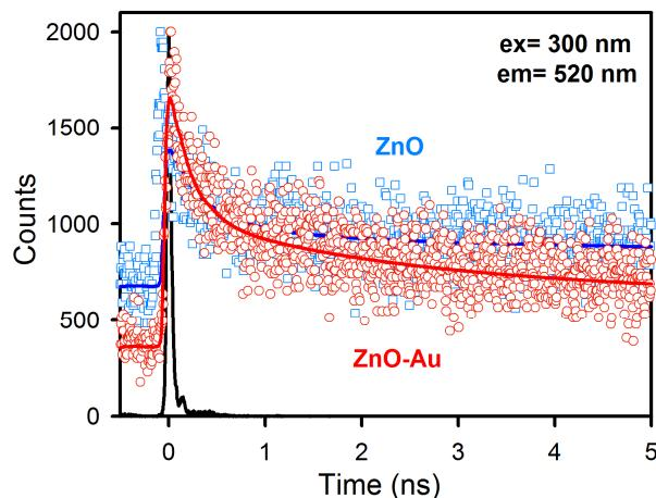
**Figure S4.** The picoseconds-resolved fluorescence transients of ZnO NPs, in the absence (blue) and presence of acceptor Au (red) (excitation at 300 nm) collected at 520 nm.
