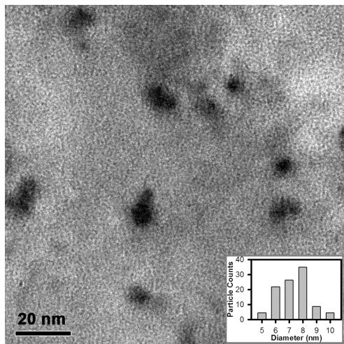
**Figure S3:** Low-Resolution TEM (LRTEM) image of ZnO-Au NCs (inset shows particle size distribution of Au NPs attached to ZnO NPs).
