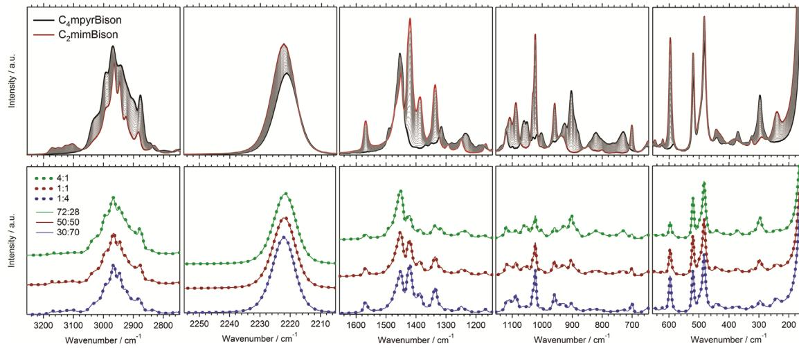
**Figure S1.** Raman spectra of  $\text{C}_2\text{mimBison}$ ,  $\text{C}_4\text{mpyrBison}$  and twenty IL linear combinations (top), and Raman spectra of three IL mixtures (4:1, 1:1, and 1:4; by volume) and the best fits of linearly combined spectra of the neat ILs (bottom).
