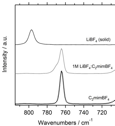
**Figure S2.** Raman spectroscopy results ( $v_s(\text{BF})$ ) from a 1M  $\text{LiBF}_4 \cdot \text{C}_2\text{mimBF}_4$  electrolyte with reference to the  $\text{LiBF}_4$  salt (top) and  $\text{C}_2\text{mimBF}_4$  ionic liquid (bottom).
