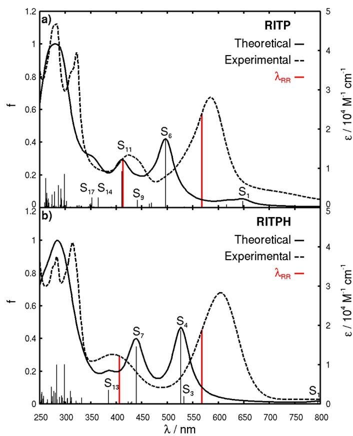
**Figure S1:** Experimental (dashed line) and theoretical (PBE0, black line) absorption spectra of the RITP and RITPH species in acetonitrile. The calculated oscillator strengths are represented by black sticks. A Lorentzian function with a half-width of 20 nm is employed to broaden the transitions in the simulated spectrum. The two vertical lines indicate the wavelengths at which the RR measurements are performed for the unprotonated (568 and 413 nm) and the protonated species (568 and 406 nm).
