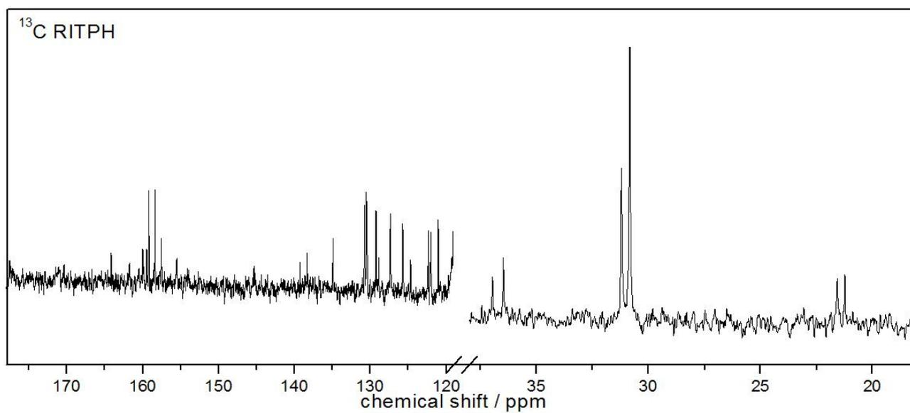
**Figure S6:** <sup>13</sup>C NMR spectrum of RITPH
