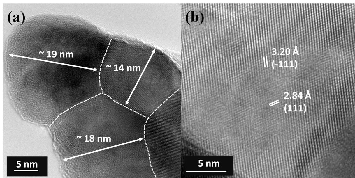
**Fig. S5** TEM images of an IBAZ  $\text{ZrO}_2$  film after an 1-hour annealing at  $1000 \text{ }^\circ\text{C}$  in air. (a) Bright field image showing the grain size estimation. (b) a zoom-in image showing the (-111) and (111) planes of a monoclinic phase  $\text{ZrO}_2$  crystallite.
