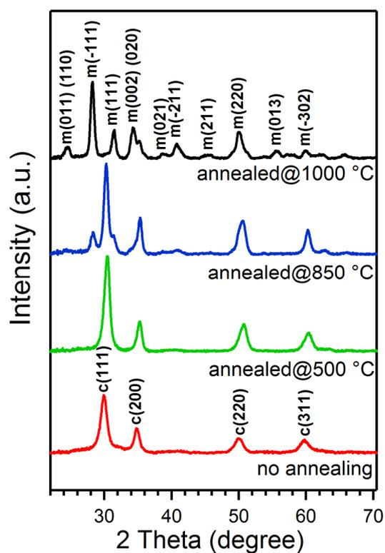
**Fig. S3** X-ray diffraction patterns of N-implanted ZrO<sub>2</sub> films without annealing and after annealing at 500 °C, 850 °C and 1000 °C. The XRD experiments were performed only for the purpose of grain size analysis. The grain sizes of these ZrO<sub>2</sub> films were estimated using the Scherrer equation as summarized in Table S1. “c” and “m” denote cubic and monoclinic ZrO<sub>2</sub>.
