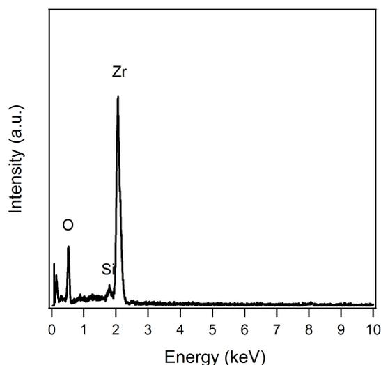
**Fig. S1** Energy dispersive spectrum of the as-synthesized nitrogen-implanted  $\text{ZrO}_2$  film.
