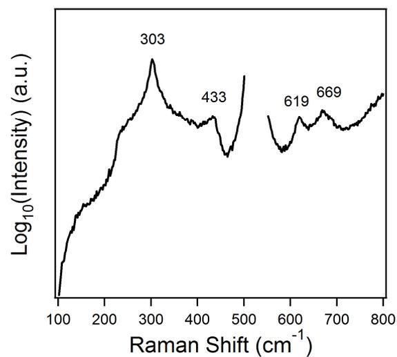
**Fig. S4** Raman spectrum of a 200-nm thick silicon nitride film deposited on a (100) silicon wafer substrate.
