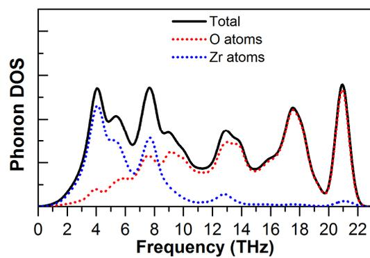
**Fig. S6** Total and partial phonon density of states for O and Zr atoms in the tetragonal ZrO<sub>2</sub>.
