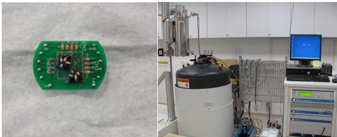
Fig.5. Device is wire bonded to the sample holder and electronic transport measurements are done by PPMS (Quantum Design).
