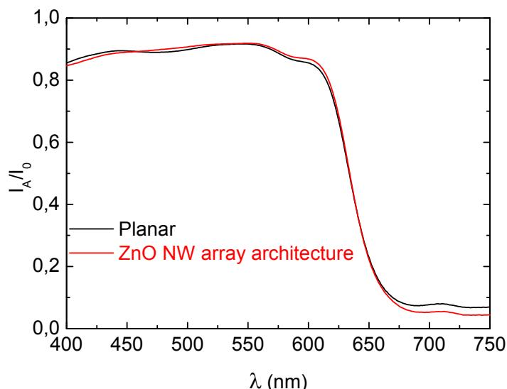
**Figure S1:** Absorbance spectra for glass/ITO/ZnO/P3HT:PCBM samples with different architectures: planar (black) and nanowire array-based (red).
