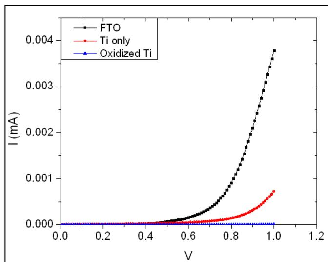
*Fig S2.* Leakage characteristics of FTO-electrolyte-FTO system vs FTO-electrolyte-titanium metal system
