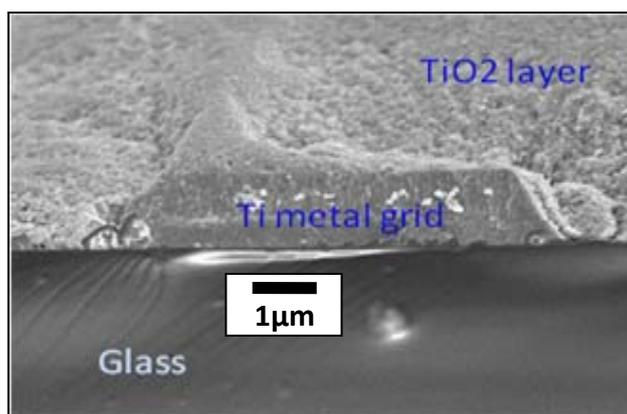
*Fig S1.* Cross section SEM image, showing that TiO<sub>2</sub> film conforms well on the metal grid
