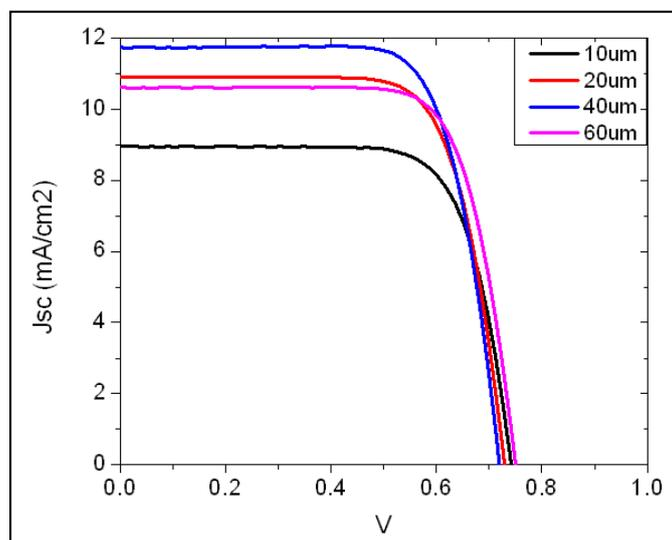
*Fig S3.* JV curves of various spacing MGE DSC (6um grid width)
