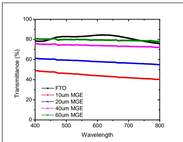
*Fig S4.* Transparency of various spacing MGE substrate (6um grid width, referenced to air)
