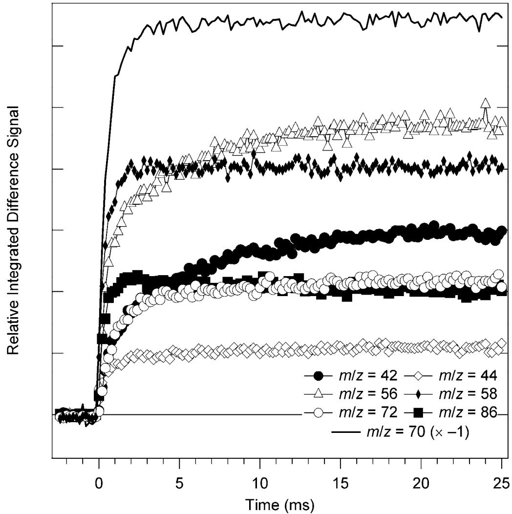
**Figure S2:** Time profiles of  $m/z = 42, 44, 56, 58, 70, 72$ , and  $86$  at  $650\text{ K}$ , obtained by integration over photon energies from  $8.0 - 10.4\text{ eV}$ . The consumption of isopentanol is shown by the profile of its daughter ion at  $m/z = 70$  (shown multiplied by  $(-1)$ ).
