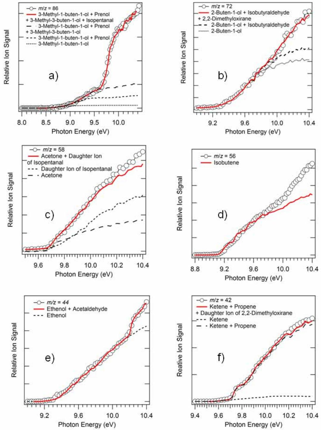
**Figure S8:** Experimental photoionization spectra and their isomeric contributions at 750 K for a)  $m/z = 86$ , b)  $m/z = 72$ , c)  $m/z = 58$ , d)  $m/z = 56$ , e)  $m/z = 44$ , and f)  $m/z = 42$ .
