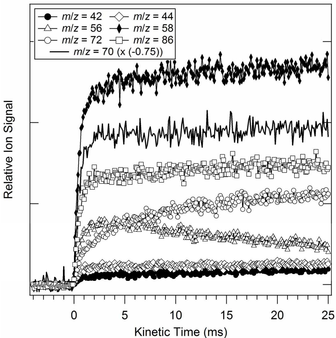
**Figure S1:** Time profiles of  $m/z = 42, 44, 56, 58, 70, 72$ , and  $86$  at  $550\text{ K}$ , obtained by integration over photon energies from  $8.0 - 10.4\text{ eV}$ . The consumption of isopentanol is shown by the profile of its daughter ion at  $m/z = 70$ , shown multiplied by  $(-0.75)$ .
