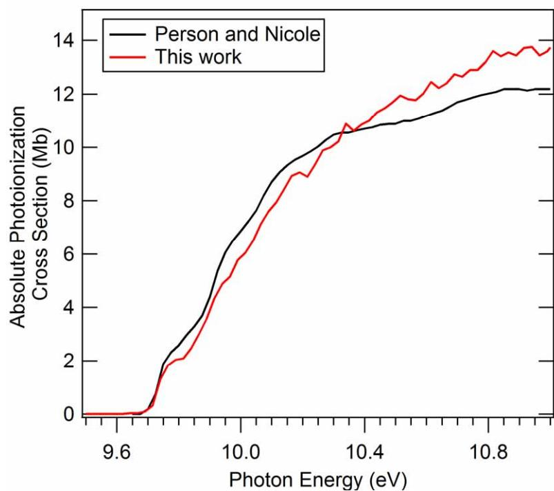
**Figure S12:** Absolute photoionization cross section of propene as reported by Person and Nicole<sup>1</sup> compared to the relative propene ion signal normalized to the photon current measured in this work. The normalized propene ion signal measured in our experiment has a different energy dependence and is scaled to match the Person and Nicole trace at 10.325 eV.
