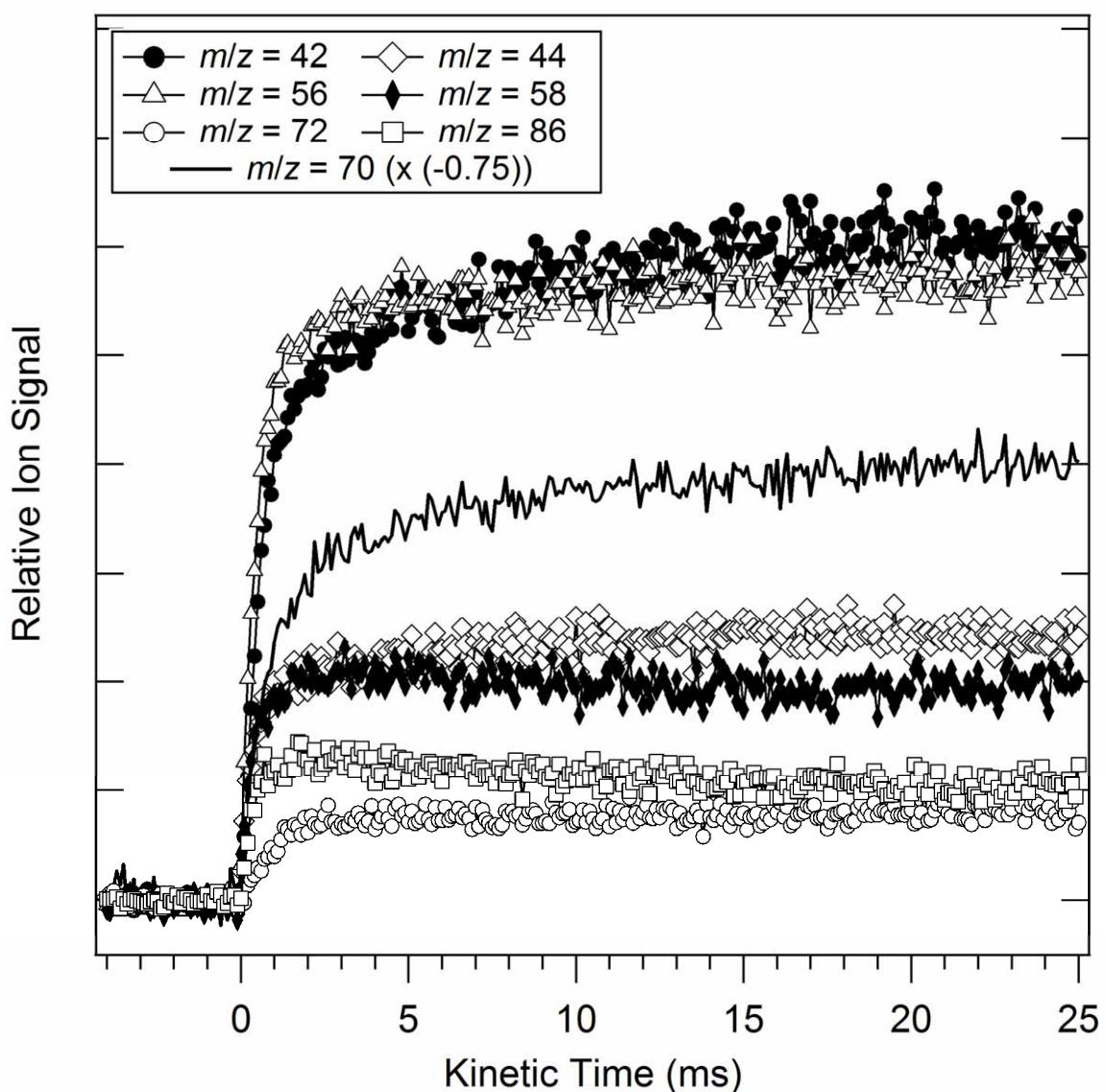
**Figure S3:** Time profiles of  $m/z = 42, 44, 56, 58, 70, 72$ , and  $86$  at  $750\text{ K}$ , obtained by integration over photon energies from  $8.0 - 10.4\text{ eV}$ . The consumption of isopentanol is shown by the profile of its daughter ion at  $m/z = 70$ , shown multiplied by  $(-0.75)$ .
