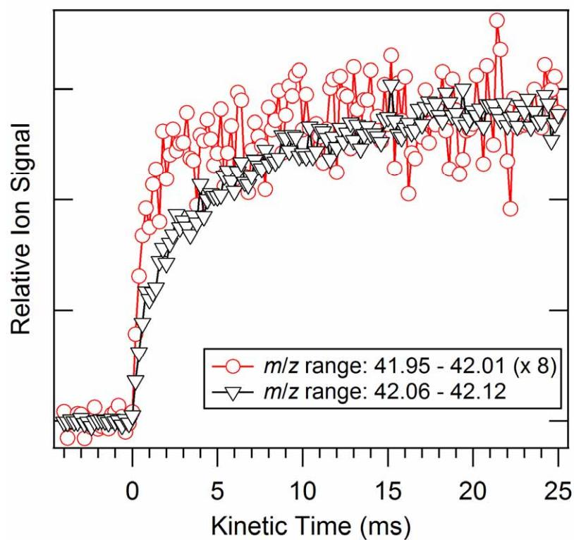
**Figure S4:** Time profiles of ketene (connected red open circles) and propene (connected black triangles) at 650 K, obtained by integrating over the mass ranges  $41.95 < m/z < 42.01$  (shown multiplied x 8) and  $42.06 < m/z < 42.12$ , respectively. The lower-mass part corresponds mostly to ketene ( $m/z = 42.01$ ), the higher-mass part mostly to propene ( $m/z = 42.05$ ). Propene shows a slower rise than ketene at longer times.
