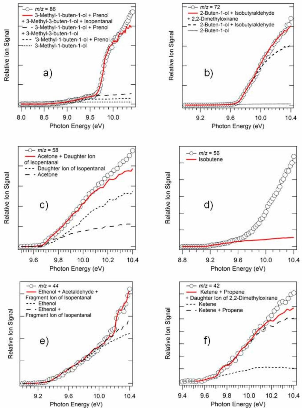
**Figure S7:** Experimental photoionization spectra and their isomeric contributions at 550 K for a)  $m/z = 86$ , b)  $m/z = 72$ , c)  $m/z = 58$ , d)  $m/z = 56$ , e)  $m/z = 44$ , and f)  $m/z = 42$ .
