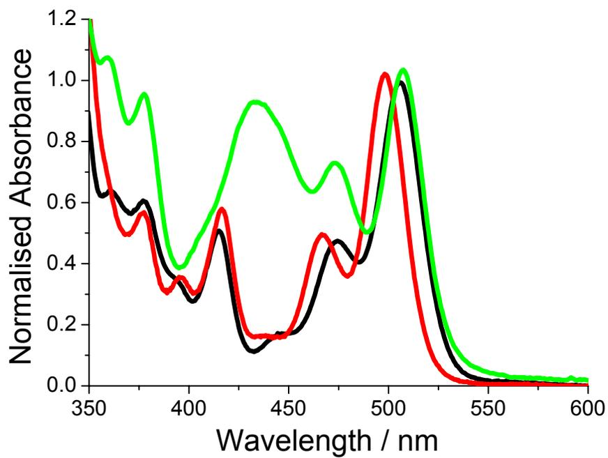
S3. Normalised absorption spectra for **1a** (red), **1b** (black) and **ACR<sup>+</sup>** (green) in dry CH<sub>3</sub>CN.
