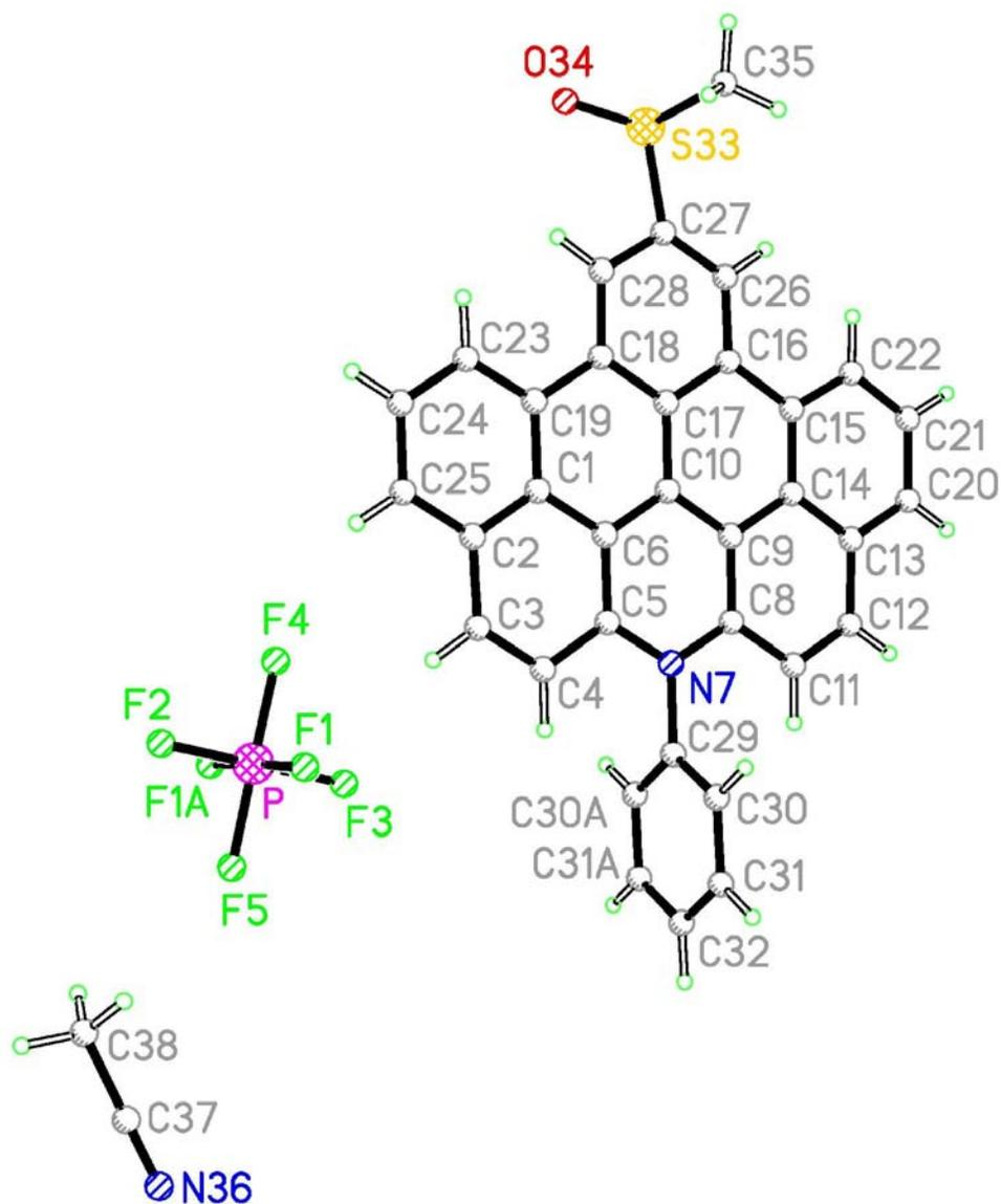
**S8.** X-ray crystallographic structure for the acetonitrile-solvated hexafluorophosphate salt of an expanded acridinium-based cation for which R = SOMe. Atoms with a suffix A are generated by crystallographic mirror symmetry. The SOMe substituent is disordered across this mirror plane, in which the whole condensed polyaromatic ring system lies. The anion and solvent molecule also lie on the mirror plane.
