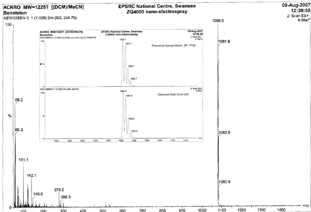
S1. Electrospray mass spectrum for ACR<sup>+</sup> and insert showing comparison of theoretical and found isotope pattern for the molecular ion.
