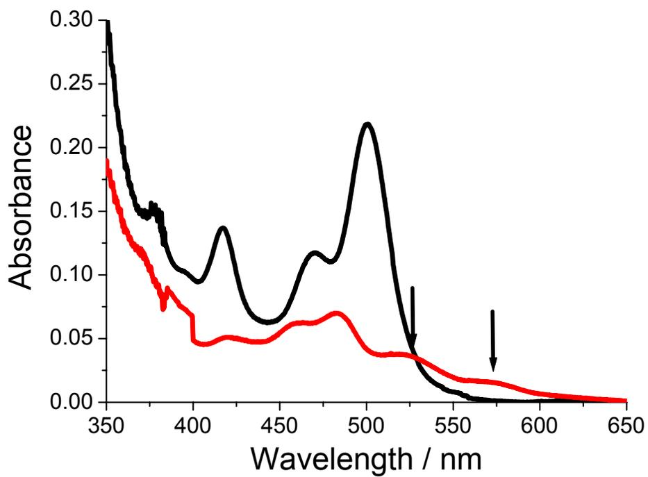
**S4.** Spectroelectrochemistry for **1a** in dry CH<sub>3</sub>CN (0.2 M TBATFB) before (black) and after reduction (red). Arrows mark the broad long-wavelength absorption bands characteristic of the mono-reduced compound.
