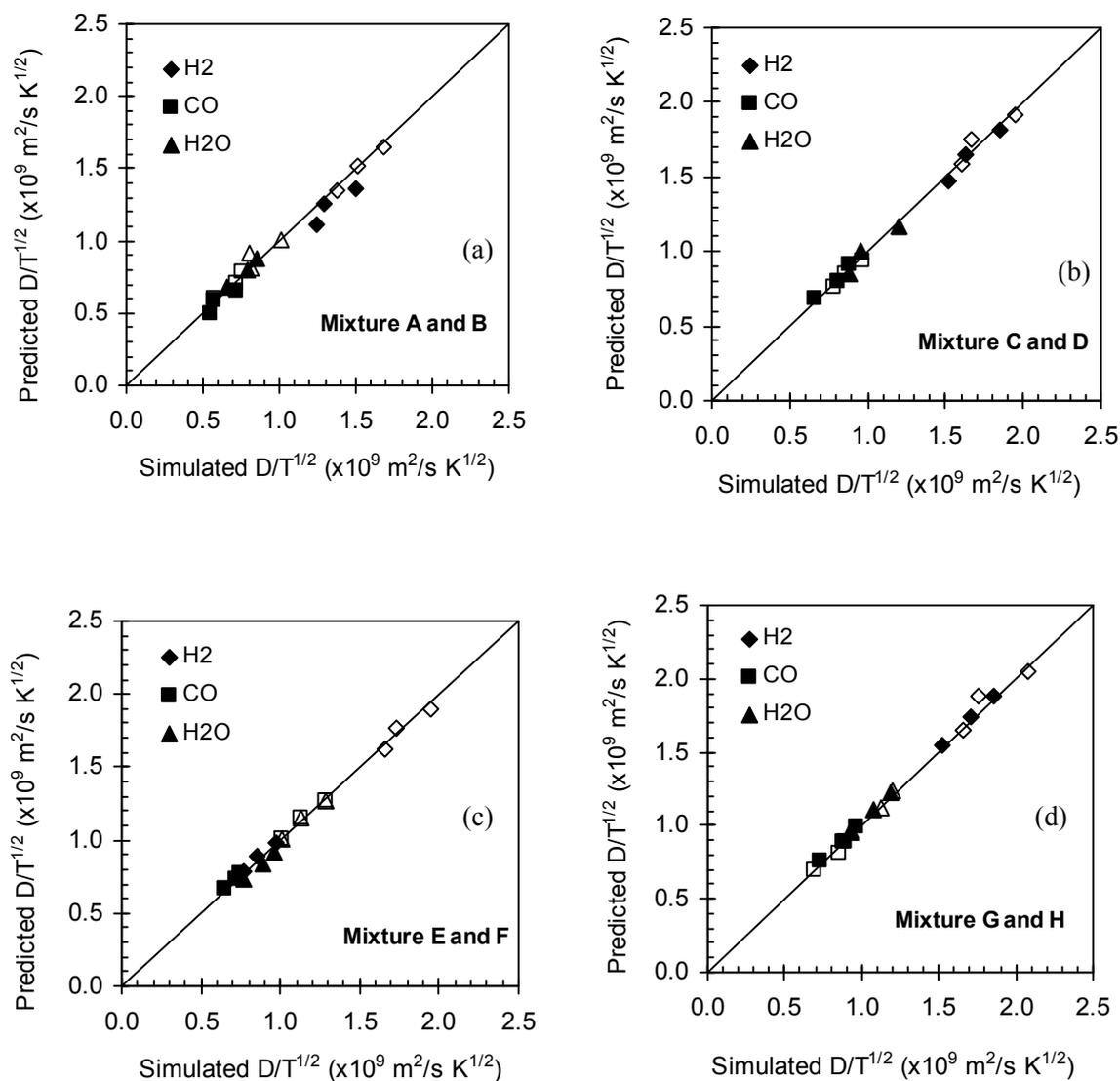
**Fig. S2.** Molecular simulation data and RHS theory correlations for the diffusivities of H<sub>2</sub>, CO and H<sub>2</sub>O in (a) mixture A (close symbols) and B (open symbols), (b) mixture C (close symbols) and D (open symbols), (c) mixture E (close symbols) and F (open symbols) and (d) mixture G (close symbols) and H (open symbols).
