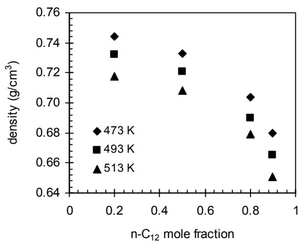
**Fig. S1.** Simulated density of  $n\text{-C}_{12}$  -  $n\text{-C}_6$  mixture as a function of  $n\text{-C}_{12}$  mole fraction.
