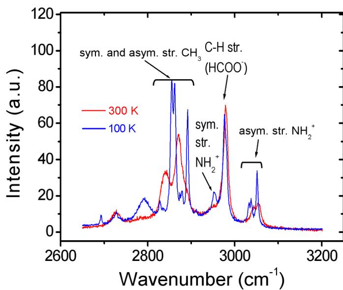
**Figure S4.** Detail of the Raman spectra results of  $[(\text{CH}_3)_2\text{NH}_2][\text{Mg}(\text{HCOO})_3]$ , corresponding to the high wavenumber region at temperature of  $T=100\text{K}$  and  $300\text{K}$ .
