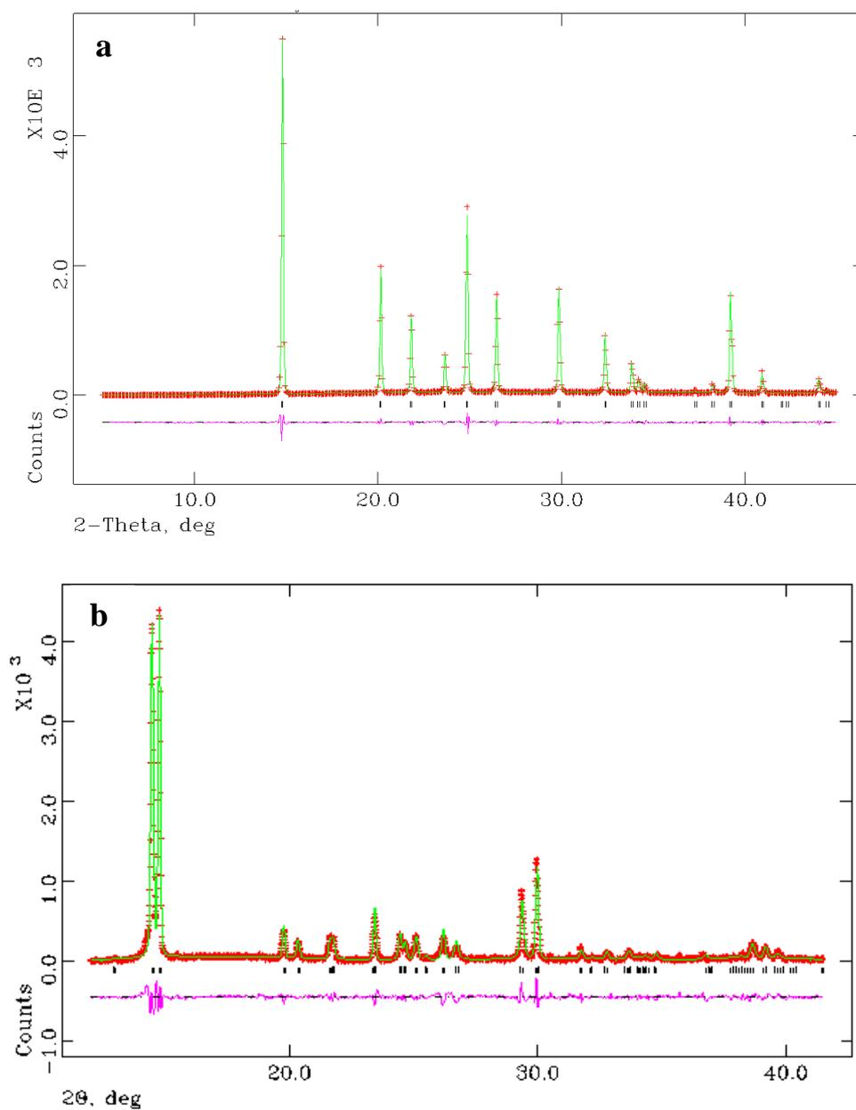
**Figure S1.** LeBail refinement of the (a) room temperature and (b) 100 K XRPD pattern. Key: observed data (+) and calculated profile (solid line); the difference plot is drawn below the profile. Tick marks indicate peak positions of the  $[(\text{CH}_3)_2\text{NH}_2][\text{Mg}(\text{HCOO})_3]$  phase.
