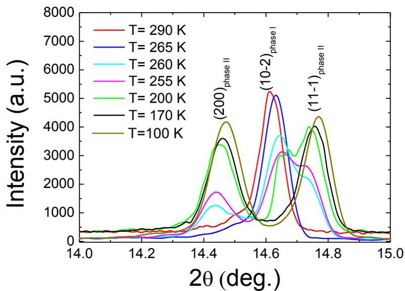
**Figure S2.** Details of the XRPD pattern obtained at different temperatures showing the structural evolution of the  $[(\text{CH}_3)_2\text{NH}_2][\text{Mg}(\text{HCOO})_3]$  compound as a function of temperature.
