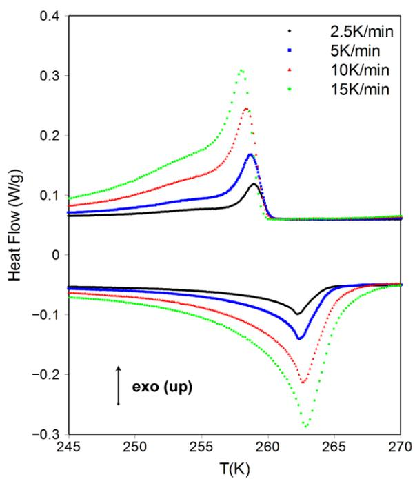
**Figure S3.** DSC results as a function of temperature obtained by heating and cooling  $[(\text{CH}_3)_2\text{NH}_2][\text{Mg}(\text{HCOO})_3]$  at different temperature rates (2.5-15 K/min).
