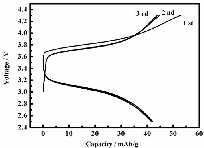
**Figure S4** Charge and discharge curves of the as-prepared Nb-doped LiFePO<sub>4</sub> sample
