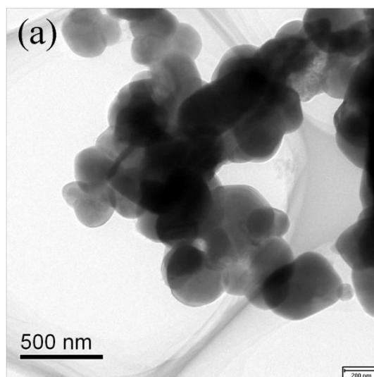
**Figure S3.** TEM image of the pristine Nb-doped LiFePO<sub>4</sub>
