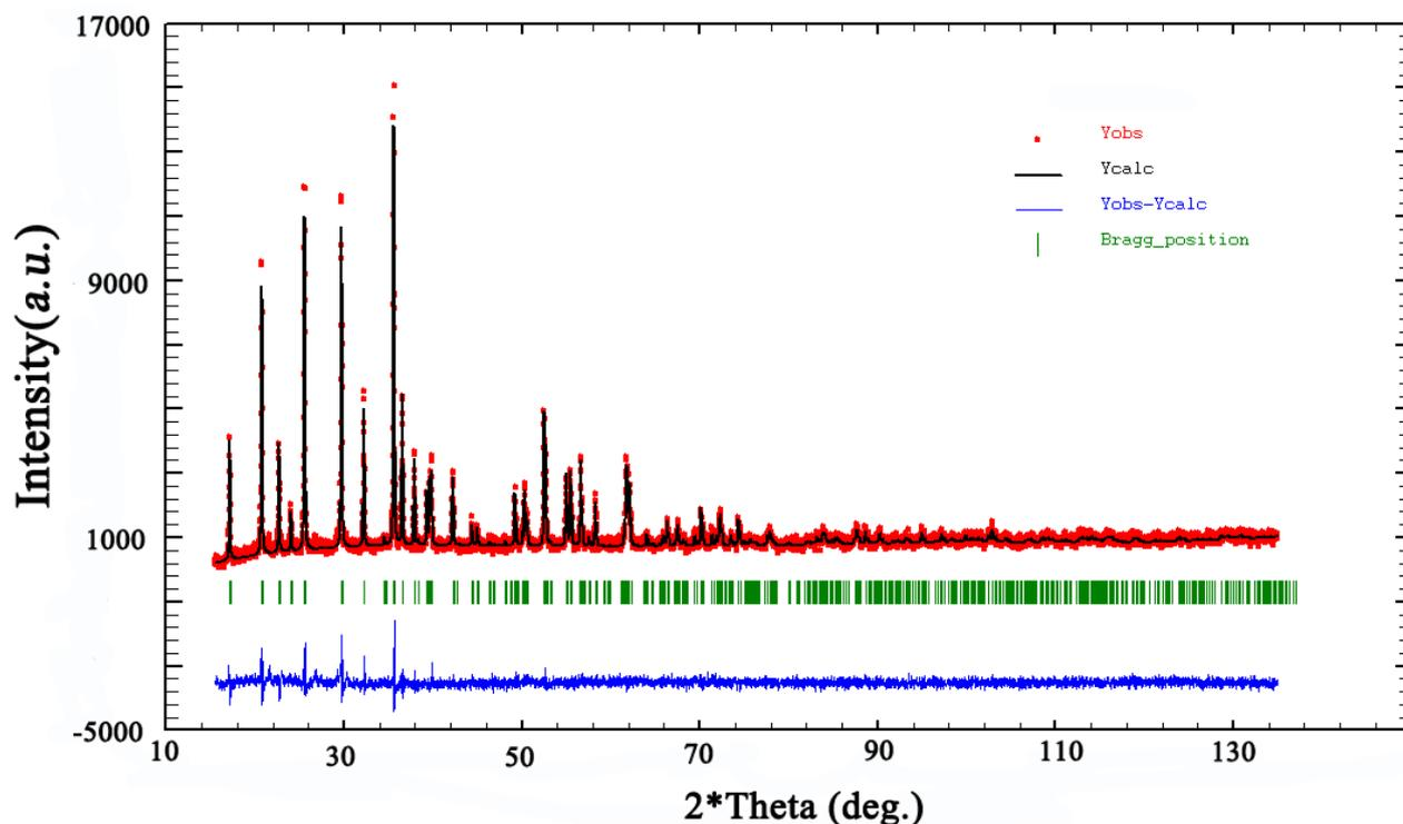
**Figure S2** Rietveld patterns of Nb-doped LiFePO<sub>4</sub> sample. Observed (red circles) and calculated (black solid line), Bragg reflection peaks (brown solid ticks) and the difference curve (below) are shown. The structural parameters are  $a = 4.6943 \text{ \AA}$ ,  $b = 10.3270 \text{ \AA}$  and  $c = 6.0048 \text{ \AA}$ ,  $R_p$ : 8.17,  $R_{wp}$ : 10.7,  $R_{exp}$ : 3.16 (not corrected for background).
