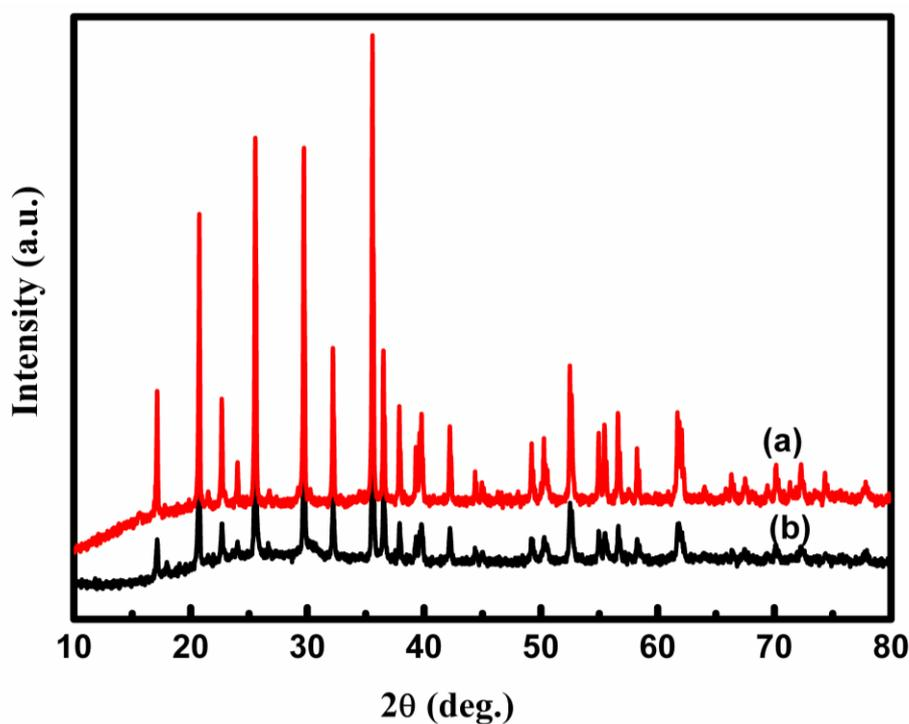
**Figure S1** XRD patterns of (a) the pristine Nb-doped  $\text{LiFePO}_4$  and (b) chemical delithiation (10 atom %)  $\text{LiFePO}_4$  sample (nominal).
