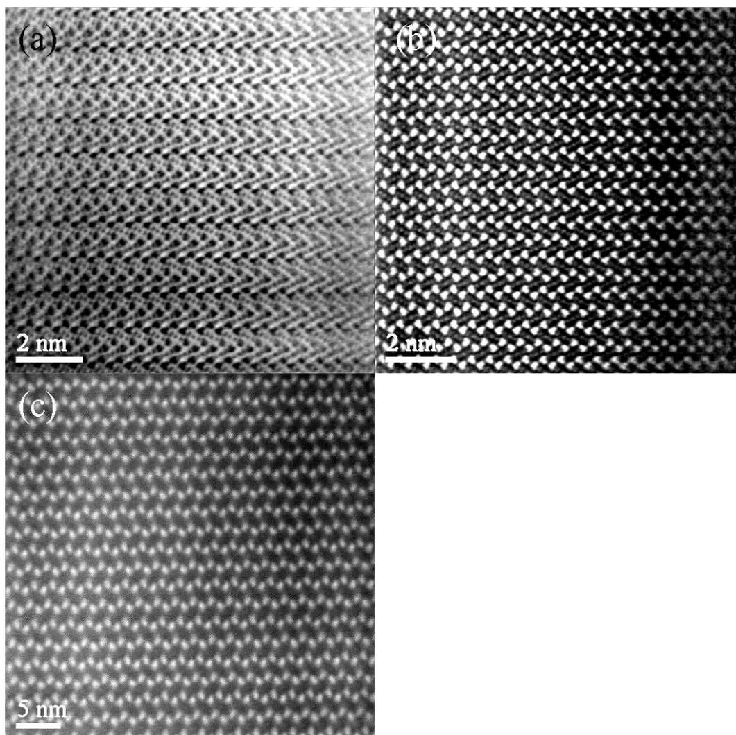
**Figure S7** Filtered STEM images of Nb-doped  $\text{LiFePO}_4$ . (a) ABF mode, (b) HADDF mode with Nb occupied in lithium site) and (c) HADDF mode with no Nb occupied in lithium site at  $[010]$  zone axis.
