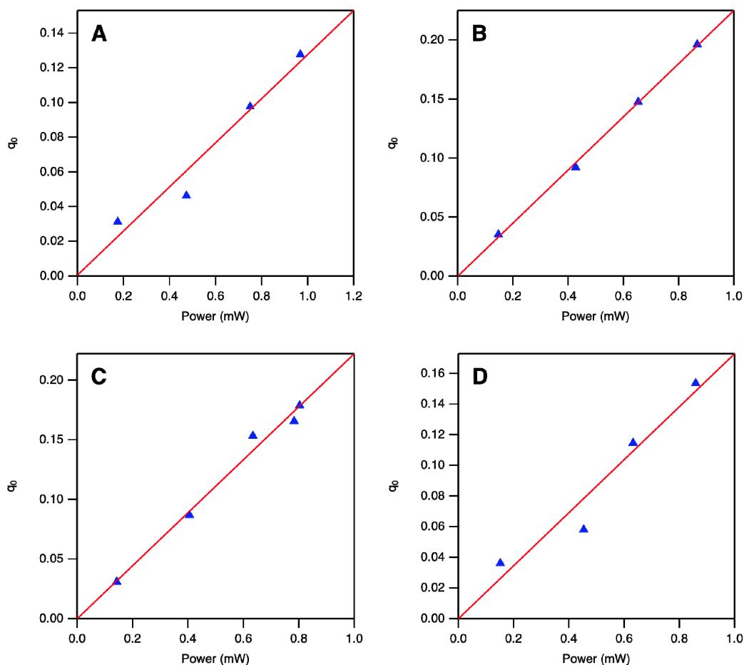
**Figure S6.** Plots of two-photon absorbance  $q_0$  of **3** in dichloromethane against the incident power at various wavelengths: 1240 nm (**A**), 1340 nm (**B**), 1445 nm (**C**), and 1550 nm (**D**). The  $q_0$  values were obtained by the curve fits in Fig. S5. The lines are linear fits to the data points.
