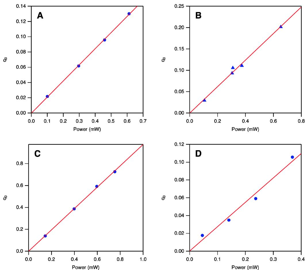
**Figure S2.** Plots of two-photon absorbance  $q_0$  of **1** in dichloromethane against the incident power at various wavelengths: 1280 nm (**A**), 1360 nm (**B**), 1590 nm (**C**), and 1520 nm (**D**). The  $q_0$  values were obtained by the curve fits in Fig. S1. The lines are
