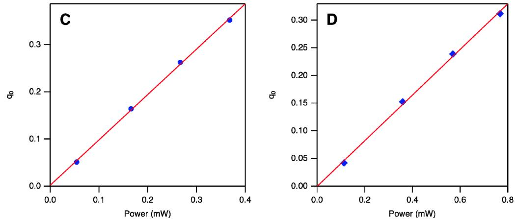
**Figure S4.** Plots of two-photon absorbance  $q_0$  of **2** in dichloromethane against the incident power at various wavelengths: 1405 nm (**A**), 1520 nm (**B**), 1590 nm (**C**), and 1680 nm (**D**). The  $q_0$  values were obtained by the curve fits in Fig. S3. The lines are linear fits to the data points.
