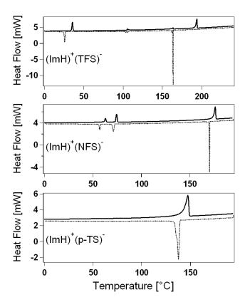
**Fig. S2** DSC plots for the thermally stable imidazole-based PICs. Solid lines: starting heating curves. Dotted lines: cooling curves.
