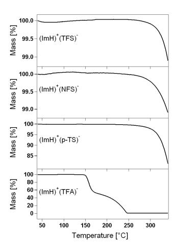
Fig. S1 Thermogravimetric curves for the imidazole-based PICs.
