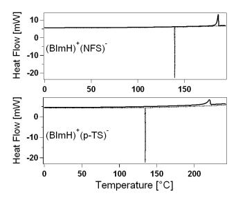
**Fig. S3** DSC plots for the thermally stable benzimidazole-based PICs (plot for sample (BimH)<sup>+</sup>(TFS)<sup>-</sup> is shown in Fig. 4 of the paper). Solid lines: starting heating curves. Dotted lines: cooling curves.
