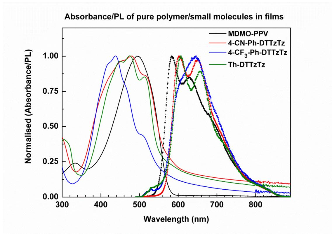
**Fig. S2** Normalized UV-vis absorption (solid curves) and PL spectra (symbols,  $\lambda_{exc} = 474$  nm) of spin-coated films of the pure compounds **MDMO-PPV** (black), **4-CN-Ph-DTTzTz** (red), **4-CF<sub>3</sub>-Ph-DTTzTz** (blue) and **Th-DTTzTz** (green).
