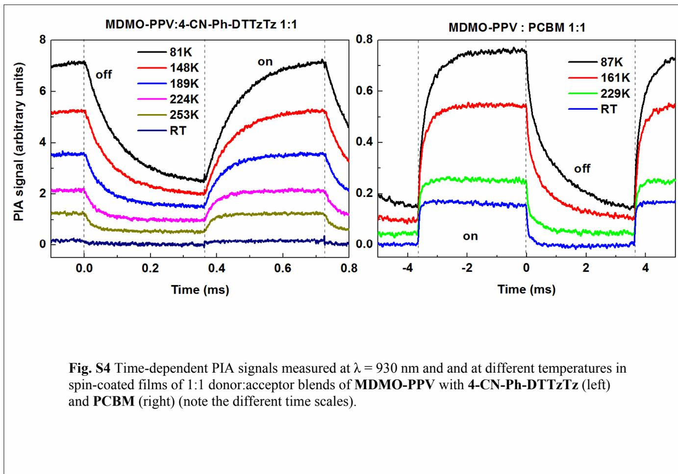
**Fig. S4** Time-dependent PIA signals measured at  $\lambda = 930$  nm and at different temperatures in spin-coated films of 1:1 donor:acceptor blends of **MDMO-PPV** with **4-CN-Ph-DTTzTz** (left) and **PCBM** (right) (note the different time scales).
