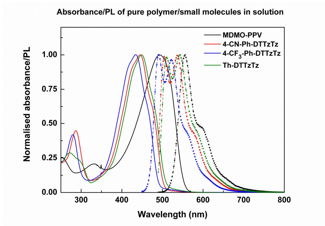
**Fig S1** Normalized UV-vis absorption (solid curves) and PL spectra (symbols) of **MDMO-PPV** (black), **4-CN-Ph-DTTzTz** (red), **4-CF<sub>3</sub>-Ph-DTTzTz** (blue) and **Th-DTTzTz** (green) in CHCl<sub>3</sub> solutions (10<sup>-5</sup> M). PL measured for  $\lambda_{\text{exc}} = 474$  nm, except for **4-CF<sub>3</sub>-Ph-DTTzTz** for which  $\lambda_{\text{exc}} = 430$  nm.
