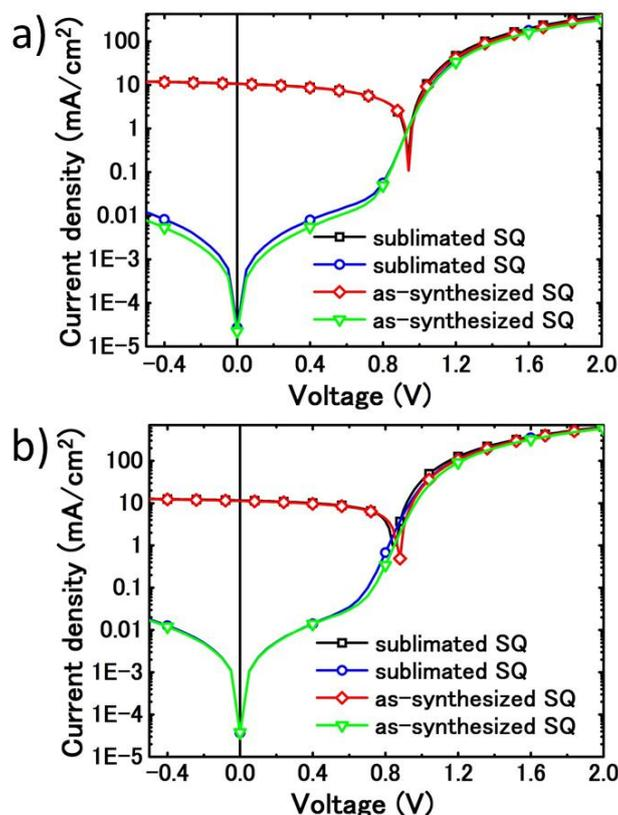
**Fig. S6** *J-V* characteristics from 1:5 SQ:PC<sub>70</sub>BM ratio cells based on as-synthesized and sublimated SQ at (a) room temperature and (b) 80 °C. It shows almost identical *J-V* characteristics and  $\eta_p$  from the PV cells based on as-synthesized and sublimated SQ.
