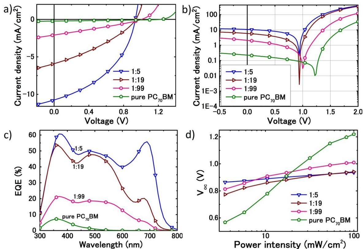
**Fig. S5** Linear (a) and logarithmic (b) *J-V* characteristics of SQ:PC<sub>70</sub>BM (1:5, 1:19, 1:99) cells and PC<sub>70</sub>BM-only cell illuminated at 100 mW/cm<sup>2</sup> of AM 1.5G; (c) EQE spectra; d) V<sub>oc</sub> vs incident light intensity.
