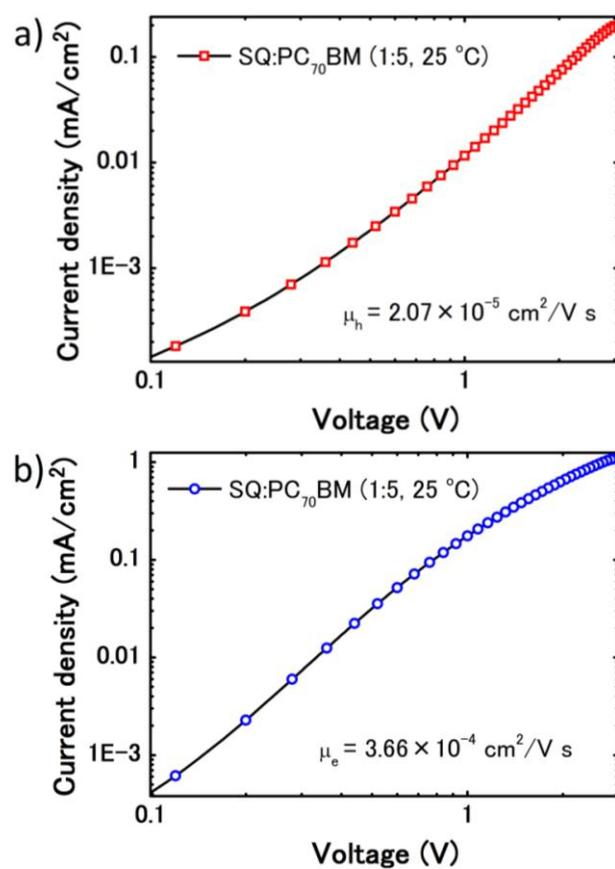
**Fig. S4** Current density vs voltage characteristic of SQ:PC<sub>70</sub>BM (1:5) single carrier devices used for a) hole and b) electron mobility measurement.
