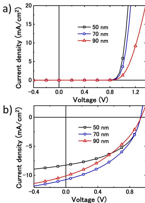
**Fig. S2** (a) Dark J-V characteristics, (b) J-V characteristics illuminated at 100 mW/cm<sup>2</sup> (AM 1.5G) for the SQ:PC<sub>70</sub>BM (1:5) BHI solar cells with varied thicknesses of the active layer.
