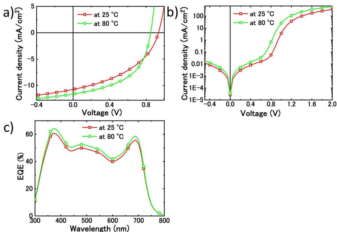
**Fig. S3** Comparison of (a) bright-state J-V characteristics; (b) dark-state J-V characteristics; (c) external quantum efficiency of SQ:PC<sub>70</sub>BM (1:5) cells at room temperature and 80 °C.
