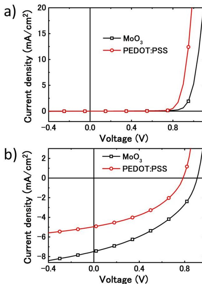
**Fig. S1** (a) Dark J-V characteristics, (b) J-V characteristics illuminated at 100 mW/cm<sup>2</sup> (AM 1.5G solar spectrum) for the SQ:PC<sub>60</sub>BM (1:5, 70nm) solar cells using MoO<sub>3</sub> and PEDOT:PSS as anode buffer layers. **Note the device data in this figure were based on PC<sub>60</sub>BM, and thus showed low photocurrent.**
