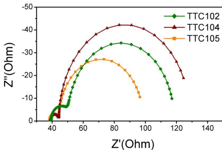
**Fig. S2** Nyquist plots of Electrochemical impedance Spectroscopy (under dark) of DSSCs based on TTC102, TTC104, and TTC105, scanned from  $10^5$  to 1 Hz. The applied potential and ac amplitude were set as -0.4 V and 10 mV, respectively.
