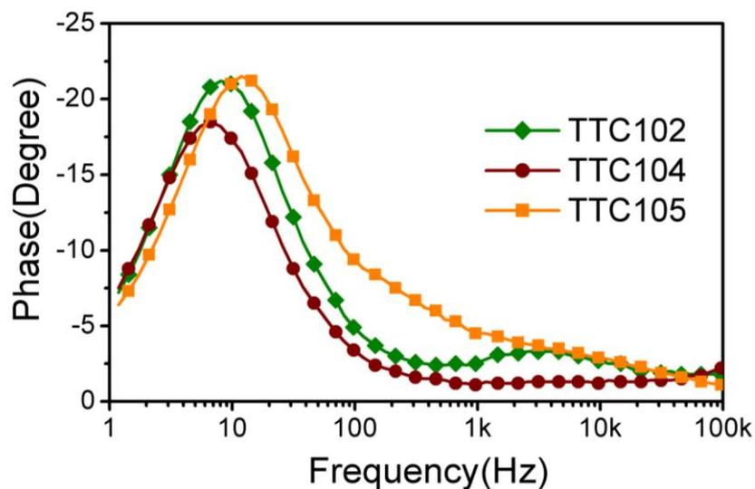
**Fig. S3** Bode phase plots of Electrochemical impedance Spectroscopy (under dark) of DSSCs based on TTC102, TTC104, and TTC105, scanned from  $10^5$  to 1 Hz. The applied potential and ac amplitude were set as -0.4 V and 10 mV, respectively.
