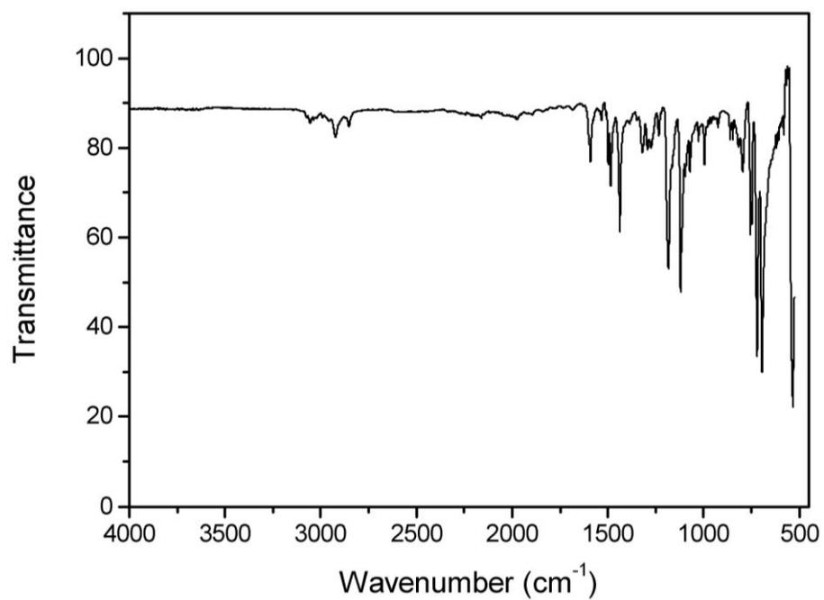
**Fig. S5** The attenuated total reflection Fourier transform infrared (ATR-FTIR) spectrum of TTC105.
