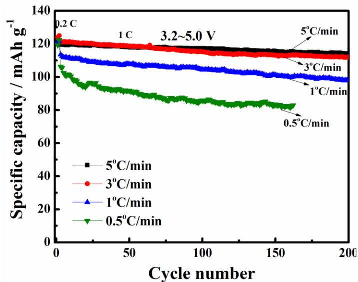
**Figure S5.** Cycling performance for  $\text{LiNi}_{0.5}\text{Mn}_{1.5}\text{O}_4$  prepared with different cooling rates at 1 C after initial charge/discharge at 0.2 C for 2 cycles. Cycling performance tests performed on duplicate  $\text{Li}/\text{LiNi}_{0.5}\text{Mn}_{1.5}\text{O}_4$  cells again demonstrates that the spinel with high cooling rate ( $5^\circ\text{C}/\text{min}$ ) shows superior cycling stability over the other spinels with lower cooling rate.
