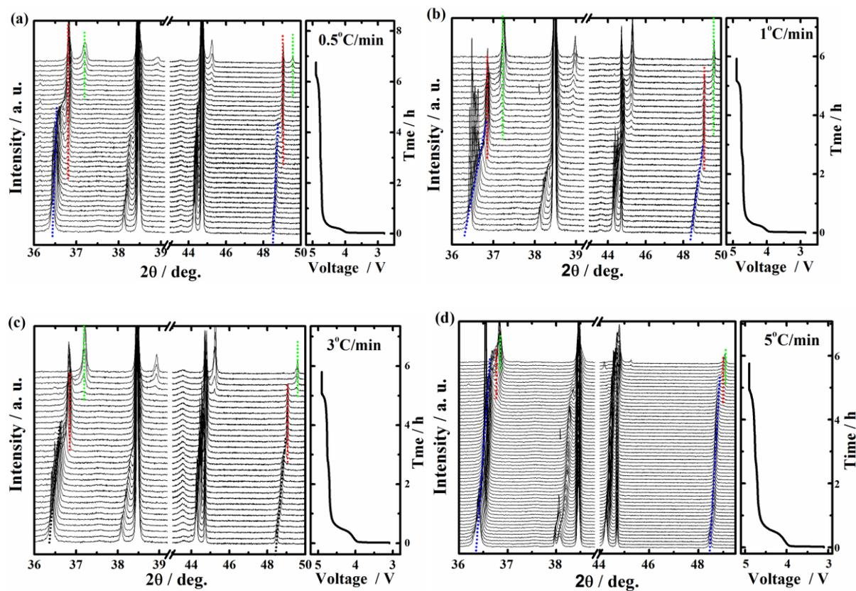
**Figure S4.** In-situ XRD patterns and corresponding charge curves of  $\text{LiNi}_{0.5}\text{Mn}_{1.5}\text{O}_4$  prepared with cooling rates of (a)  $0.5^\circ\text{C}/\text{min}$ ; (b)  $1^\circ\text{C}/\text{min}$ ; (c)  $3^\circ\text{C}/\text{min}$  and (d)  $5^\circ\text{C}/\text{min}$ . The faster cooled spinel has more disordered phase/ $\text{Mn}^{3+}$  in the lattice and longer range of solid solution reaction during initial charge processes.
