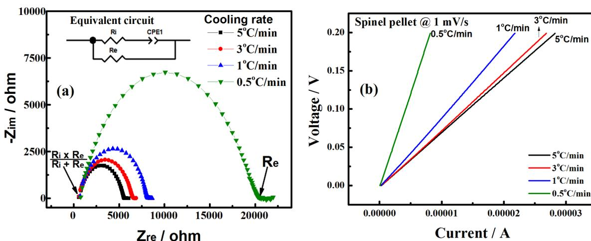
**Figure S1.** (a) Nyquist plots and (b) V/I curves of LiNi<sub>0.5</sub>Mn<sub>1.5</sub>O<sub>4</sub> pellets prepared with different cooling rates. The inset is the equivalent circuit for mixed conductive materials. Detailed parameters of pellets for conductivity test and results of the ionic and electronic conductivities are shown as follows. Electronic conductivities measured by two methods are consistent.
