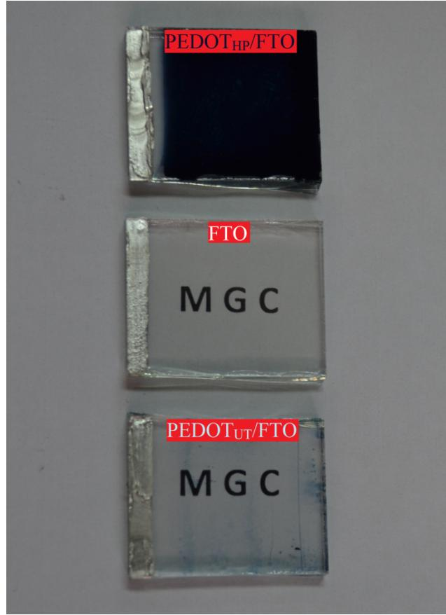
**Fig. S3** Digital photographs of PEDOT<sub>HP</sub> coated FTO and PEDOT<sub>UT</sub> coated FTO glasses.
