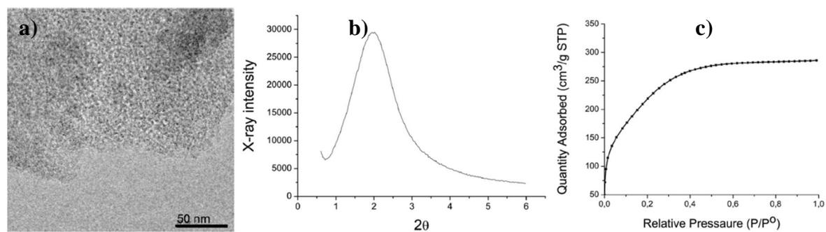
**Fig. S1:** Characterization of mesoporous silica particles. a) A representative transmission electron microscope image; b) the X-ray diffraction spectra; and c) the nitrogen isotherm of the calcined mesoporous particles.
