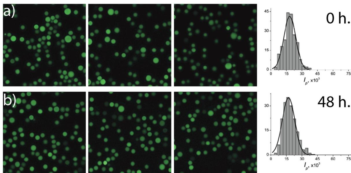
**Fig. S3:** CLSM images of mesoporous silica particles loaded with Sodium Green and sealed with DLPC lipid bilayer without gramicidin A. Panel shows three representative-CLSM images and the histograms of the integral intensity per particle a) before and b) 48 h. after injection of  $\text{Na}^+$  to the outer bulk solution. CLSM images of optical sections at particles equator in each panel were recorded keeping the experimental conditions, microscope hardware and software settings identical.
