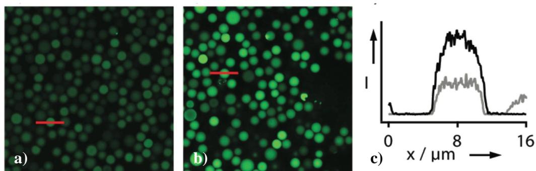
**Fig. S2:** CLSM scans of particles without lipid bilayers sealing before and after Na<sup>+</sup> uptake. Images a) and b) corresponds to the two extreme cases of 0 mM and 100 mM of Na<sup>+</sup> inside particles, respectively, preloaded with the same concentration of SG. Graph c) is an intensity plot across representative particles along red lines in a) and b).
