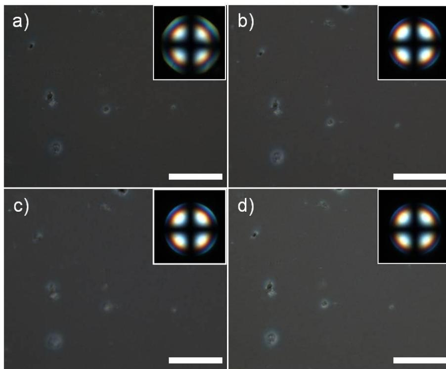
**Figure S5.** POM images of identical homeotropic region of 5CB containing 0.001 wt% SWNT upon arresting temperature in N phase for (a) 24 hours, (b) 48 hours, (c) 72 hours and (d) 96 hours. Insets show corresponding Bertrand interference pattern from identical region for 96 hours. Images were taken under crossed polarizers. (All scale bar: 200  $\mu\text{m}$ )
