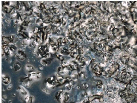
**Figure S2.** POM image of co-existence of homeotropic and planar texture of 5CB when a 100 $\mu$ m thickness cell was exposed to a 230 gauss magnetic field normal to the substrate
