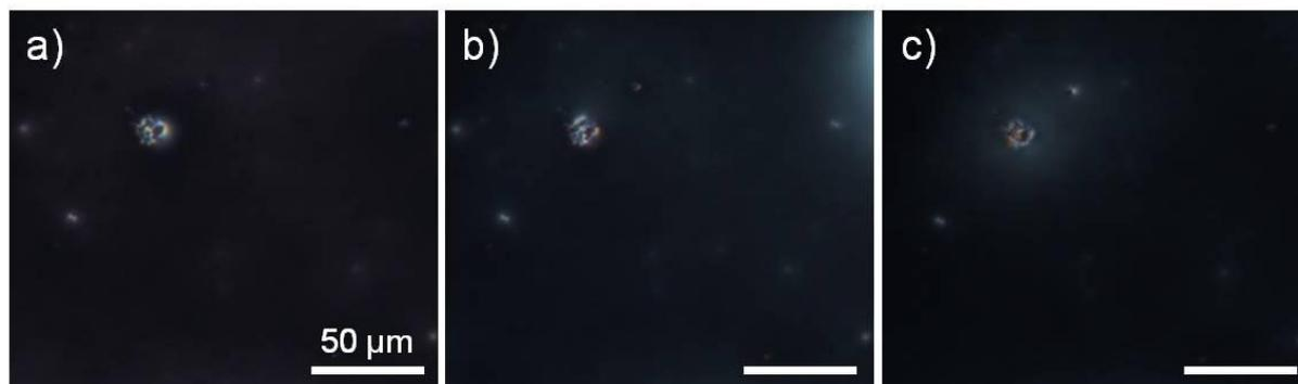
**Figure S4.** POM images of identical planar region (a-c) of 5CB. The sample was arrested above  $T_{iso}$  for 5 min and subsequently cooled to N phase: (a) 1st, (b) 2nd and (c) 3rd round of heating and cooling. All Images were taken under crossed polarizers. (All scale bar: 50 $\mu$ m)
