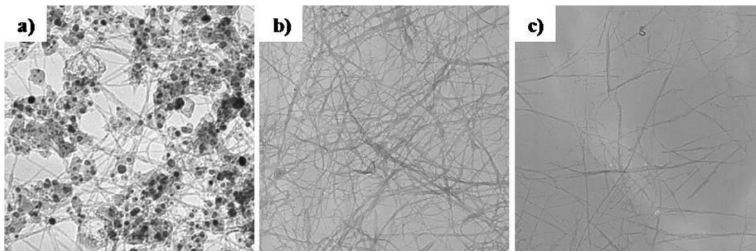
**Figure S1.** TEM images of (a) As prepared SWNTs, (b) purified SWCNTs, (c) cut SWCNTs.
