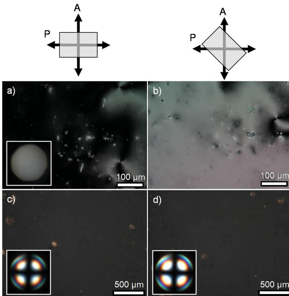
**Figure S3.** POM images of planar- (a, b) and homeotropic (c, d) alignment of 5CB by field-oriented SWNTs (0.05 wt%). The sample was rotated by  $45^\circ$  between crossed polarizers (b, d). Insets show Bertrand interference pattern for each corresponding alignments.
