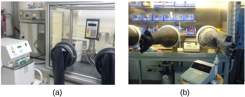
Figure S.9: Pictures of the used equipments for (a) viscosity and (b) conductivity measurements.
