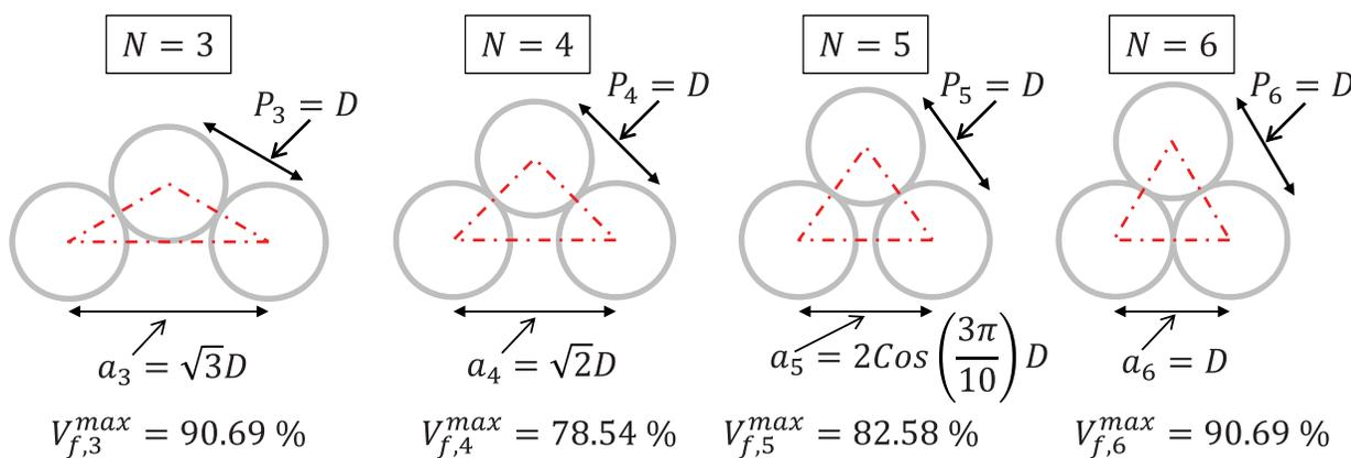
**Fig. S1** Illustration of component triangles for each coordination at the maximum theoretical volume fractions (wire walls are touching). Since the unit cell inter-wire spacing,  $S_N$ , is zero in this case,  $P_N$ , is equal to the wire diameter,  $D$ , in all coordinations.
