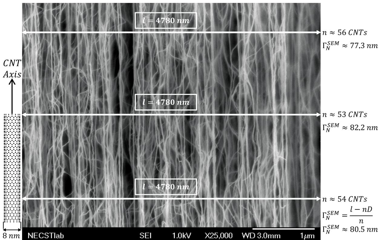
**Fig. S3** HRSEM micrograph for a 1.0 volume % CNT forest with lines drawn perpendicular to the CNT primary axis. The average inter-CNT spacing in the forest was then determined by counting only the bright in-focus CNTs underneath each line.
