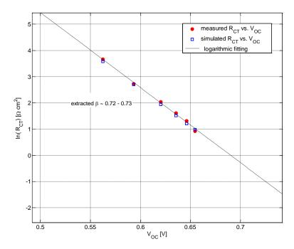
Figure S1 Comparison between recombination resistance  $R_{CT}$  as extracted, through equivalent circuit fitting, from EIS measurements and EIS simulated data. The slope provides an estimation of the exponent ( $\beta$ ) of the nonlinear recombination term in close agreement with the value estimated from the analysis of the discrepancy between IPCE and I-V as outlined in the paper.
