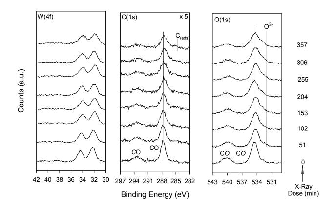
**SI 1:** Evolution of the W(4f), C(1s), and O(1s) XP regions for a 1.5nm thick film of W(CO)<sub>6</sub> irradiated with X-rays (Mg K $\alpha$  1253.6 eV); the x-ray exposure time is shown on the right hand side of each W(4f), C(1s), and O(1s) spectrum.
