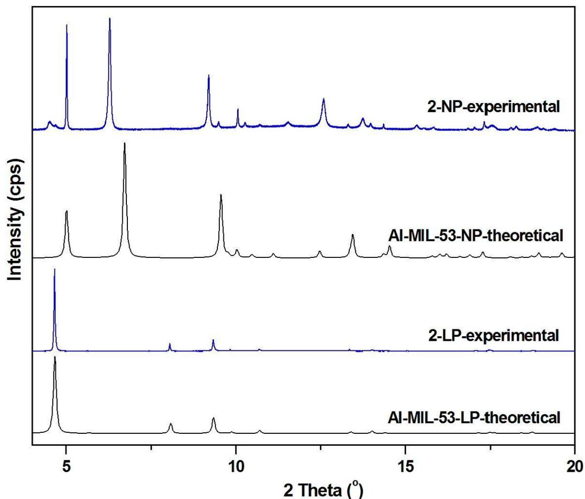
**Figure S9.** Theoretical (black) and experimental (blue) synchrotron XRPD patterns ( $\lambda = 0.827131 \text{ \AA}$ ) of the different forms of **2** and Al-MIL-53. The XRPD patterns for the LP and NP phases of **2** were collected at  $80 \text{ }^\circ\text{C}$  immediately after evacuation and after 5 h of staying under vacuum, respectively.
