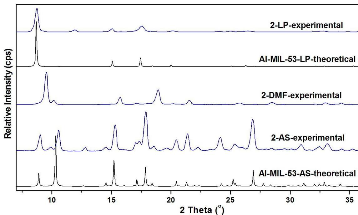
**Figure S5.** Theoretical (black) and experimental (blue) laboratory XRPD patterns ( $\lambda = 1.5406 \text{ \AA}$ ) of the different forms of **2** and Al-MIL-53.
