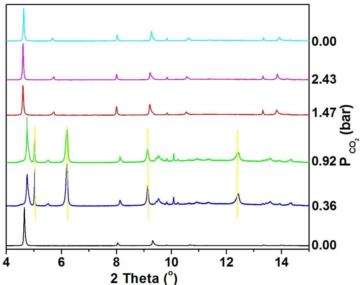
**Figure S8.** In-situ synchrotron XRPD patterns ( $\lambda = 0.827131 \text{ \AA}$ ) of **2** collected at a certain pressure of CO<sub>2</sub> and 40 °C. The Bragg peaks marked by yellow lines indicate the narrow pore phase, whereas the rest of the Bragg peaks denote the large pore phase. Before the measurement, the sample was degassed at 200 °C for 30 min under vacuum.
