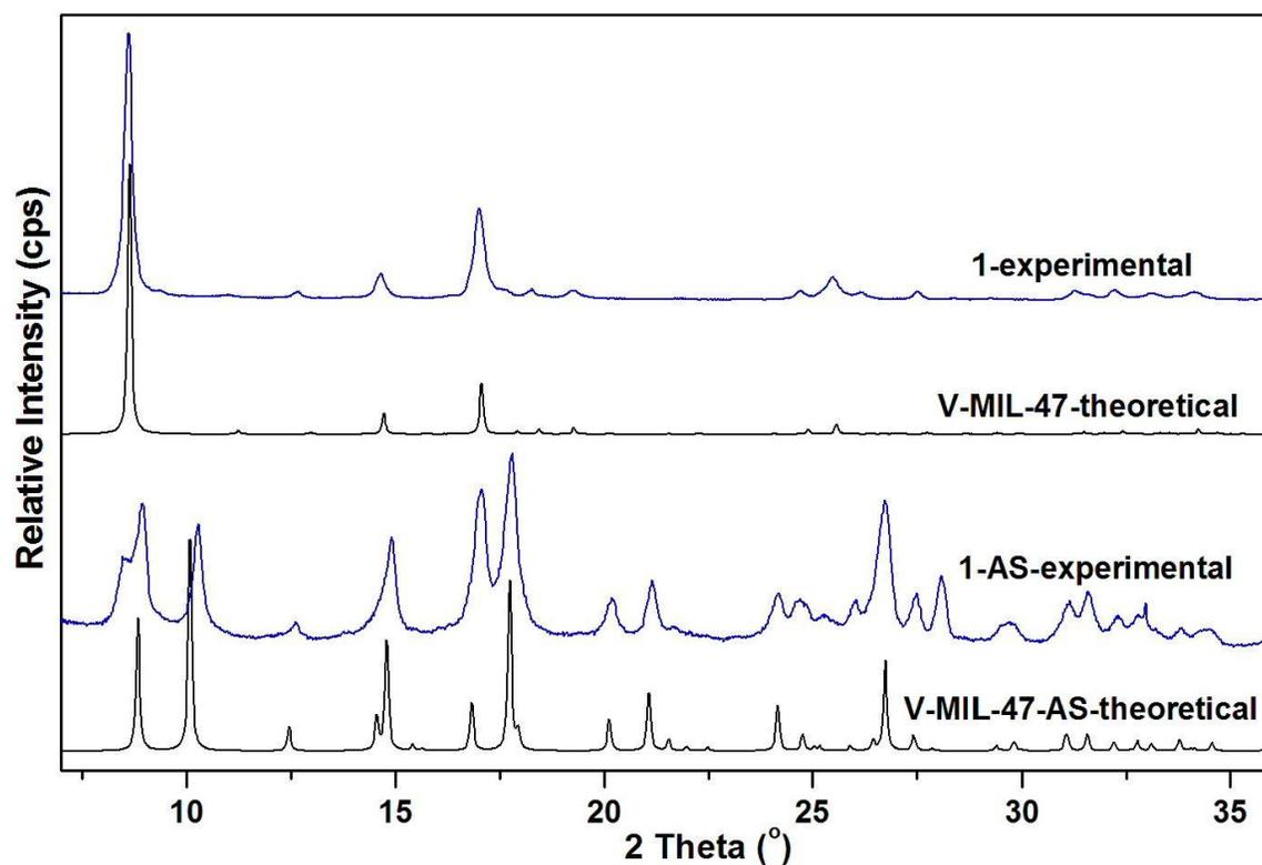
Figure S4. Theoretical (black) and experimental (blue) laboratory XRPD patterns ( $\lambda = 1.5406 \text{ \AA}$ ) of the different forms of **1** and V-MIL-47.
