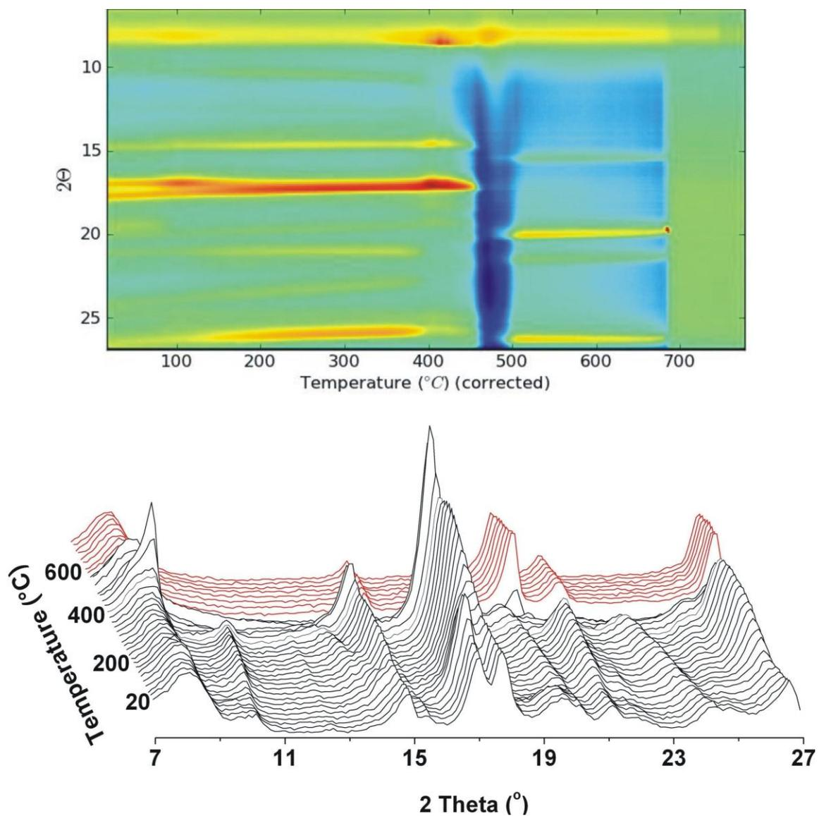
**Figure S6.** TDXRPD patterns ( $\lambda = 1.5406 \text{ \AA}$ ) of **1-AS** measured in air atmosphere in the range of 20–800 °C. The black and red patterns denote stable and decomposed phases, respectively. The variation of the intensities of the Bragg peaks as a function of temperature is shown on the top.
