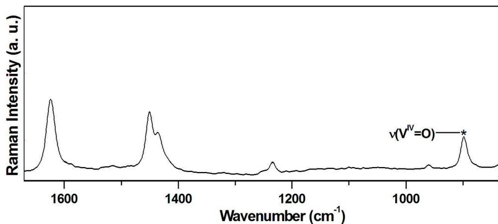
Figure S3. Raman spectrum of thermally activated **1**.
