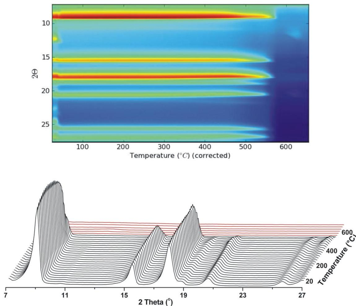
**Figure S7.** TDXRPD patterns ( $\lambda = 1.5406 \text{ \AA}$ ) of the thermally activated form of **2** measured in air atmosphere in the range of 20–650 °C. The black and red patterns denote stable and decomposed phases, respectively. The variation of the intensities of the Bragg peaks as a function of temperature is shown on the top.
