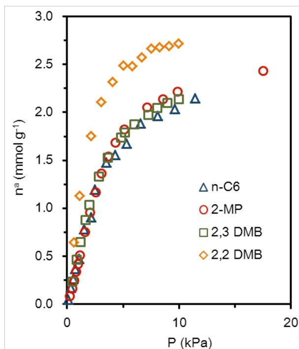
**Fig. S2** - Molecular Simulation of the hexane isomers adsorption isotherms, without blocking, on ZIF-8, at 373 K:  $\triangle$  n-hexane,  $\circ$  2-methylpentane,  $\square$  2,3-dimethylbutane, and  $\diamond$  2,2-dimethylbutane. Zoom of Figure 7a.
