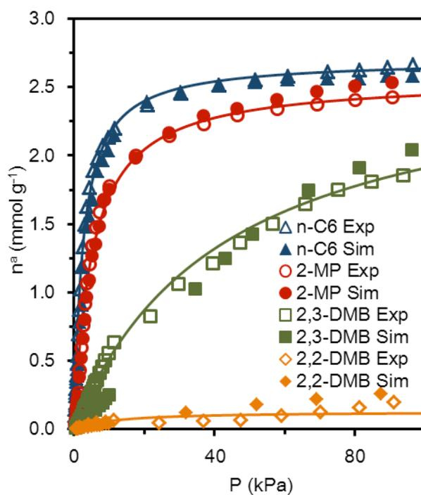
**Fig. S3** - Comparison between Experimental and Molecular Simulation hexane isomers adsorption isotherms, on ZIF-8, at 373 K:  $\triangle$  n-hexane,  $\circ$  2-methylpentane,  $\square$  2,3-dimethylbutane, and  $\diamond$  2,2-dimethylbutane.
