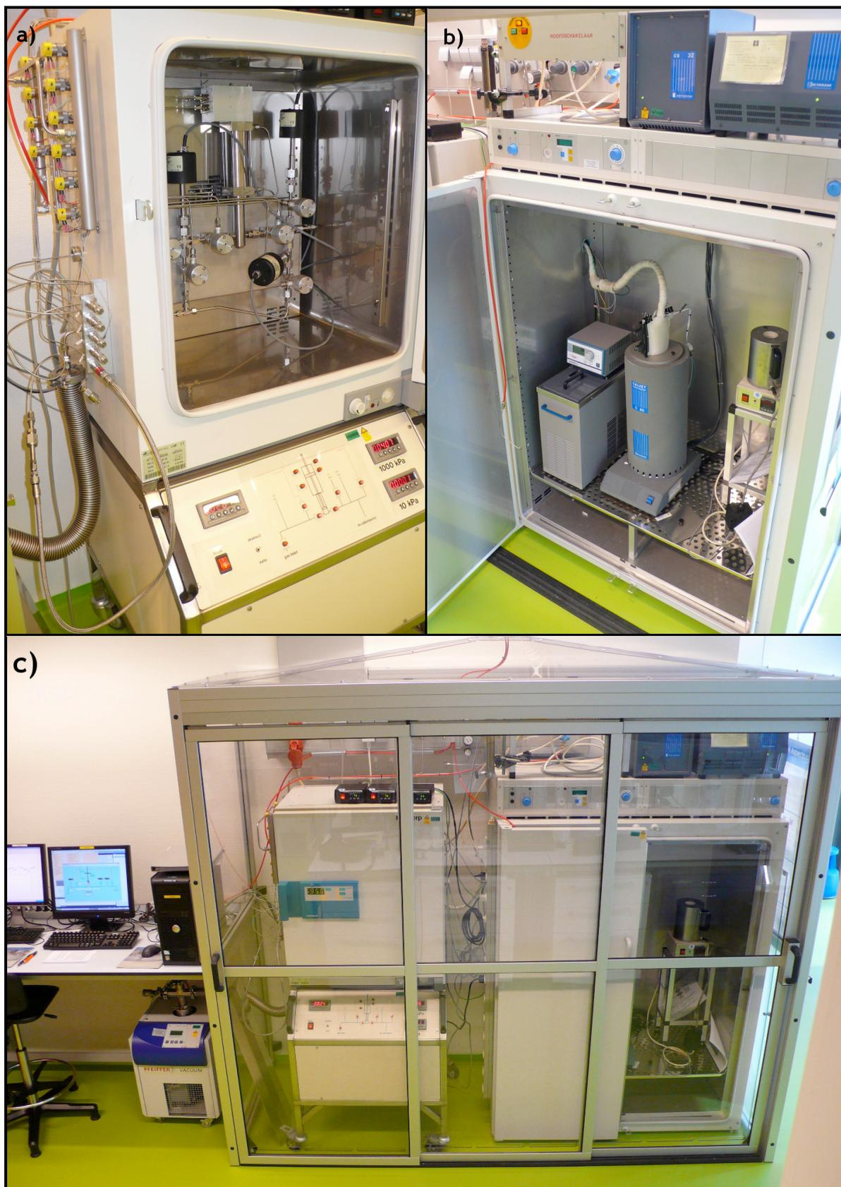
**Fig. S4** - Photograph of the experimental Set-Up: a) the volumetric introduction system, b) microcalorimeter in a thermostatic oven, and c) general over view of the connection between the two parts of the experimental system.
