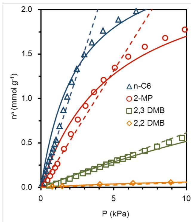
**Fig. S1** - Hexane isomers adsorption isotherms, on ZIF-8, at 373 K:  $\triangle$  n-hexane,  $\circ$  2-methylpentane,  $\square$  2,3-dimethylbutane, and  $\diamond$  2,2-dimethylbutane. Full lines are the isotherm model fits by Langmuir model (eq. 1); dashed lines are the isotherms fits by Henry Law model (eq. 2).
