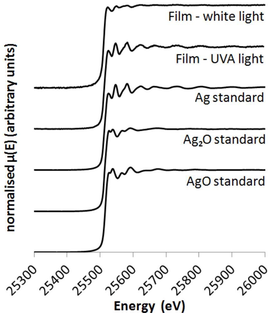
Supplementary Information 4: The full spectrum of normalized EXAFS spectra ( $\mu(E)$ ) at the K-edge of silver. Shown are AgO and Ag<sub>2</sub>O powder pellets diluted in BN (AgO and Ag<sub>2</sub>O standards), Ag foil (Ag standard) and the Ag-TiO<sub>2</sub> thin-film after being exposed to white light (Film – white light) or UVA light (Film – UVA light) for 12 hours
