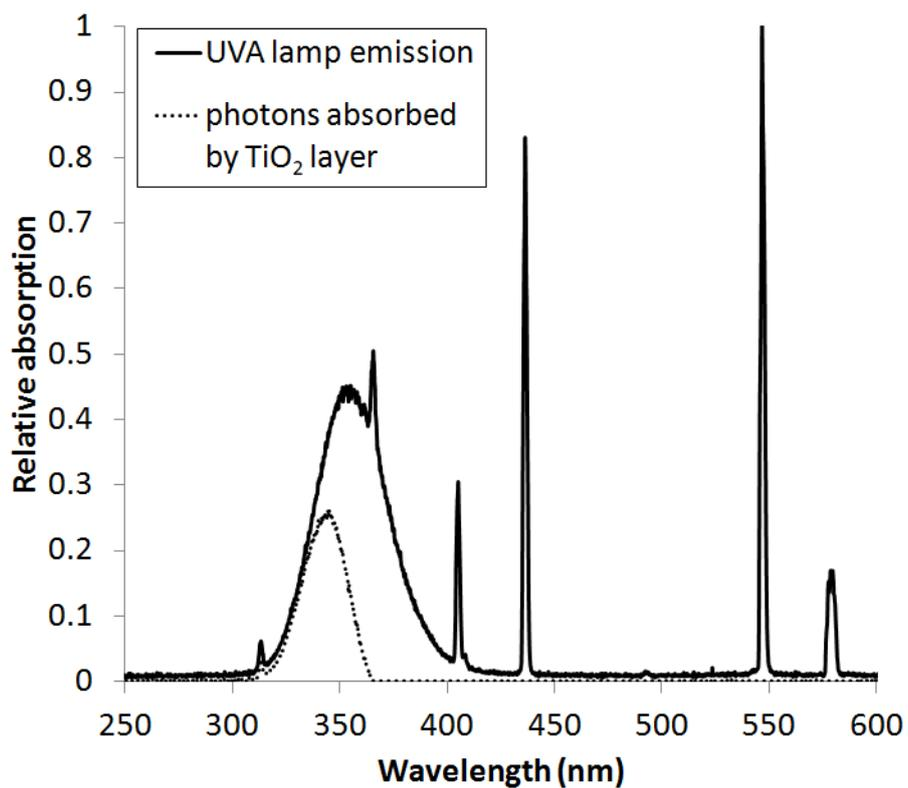
Supplementary Information 2: The emission profile of the UVA – 365 nm lamp (solid line) and the portion that was absorbed by the TiO<sub>2</sub> film (dashed line).
