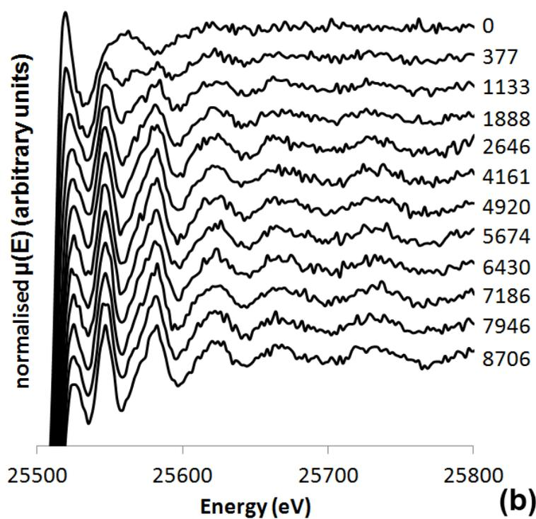
Supplementary Information 5: Stacked plots of the normalized EXAFS patterns ( $\mu(E)$ ) from the K-edge of silver during the photo-assisted growth of Ag nanoparticles from  $\text{AgNO}_3$  on  $\text{TiO}_2$  thin-films using (a) UVC ( $1.13 \times 10^{15}$  photons  $\text{cm}^{-2}\text{s}^{-1}$ ) and (b) UVA ( $2.83 \times 10^{15}$  photons  $\text{cm}^{-2}\text{s}^{-1}$ ) sources. Each pattern represents a cumulative irradiation time in seconds from which the mid-data point was measured.
