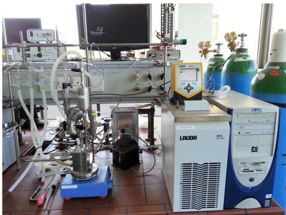
Figure 2. Photocatalytic setup for stirred dispersions.
