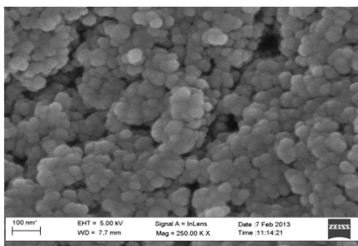
**Figure S6:** SEM image of a representative *nc*-TiO<sub>2</sub> film
