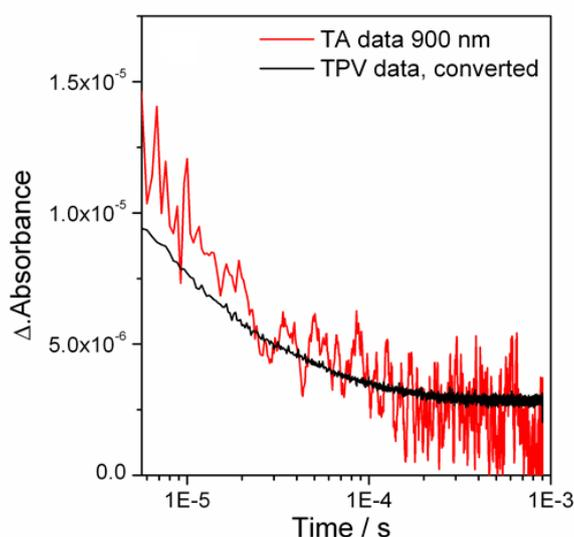
**Figure S4.** TA decay trace and TPV decay trace recorded following the UV excitation (355 nm,  $16 \mu\text{J cm}^{-2}$ ) of a *nc*-TiO<sub>2</sub> film under LED illumination (365 nm) at open circuit (-310 mV). TA data is recorded by probing the decay of the transient at 900 nm and is then converted to an equivalent change in photo voltage by use of the extinction coefficient derived in the main text.
