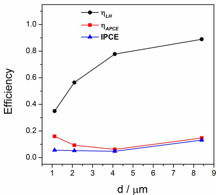
Fig S2. Dependence of IPCE,  $\eta_{LH}$  and APCE ( $\equiv (\eta_{col} \times \eta_{sep})$ ) as a function of  $nc\text{-TiO}_2$  film thickness ( $d$ ). The steady state IPCE data is recorded for a  $nc\text{-TiO}_2$  electrode illuminated (355 nm) on the electrolyte (EE) side in 0.5 M  $\text{NaClO}_4$  aqueous solutions ( $\text{pH}=2.0$ ) held at 0.6 V versus Ag/AgCl.
