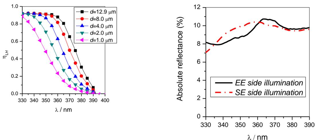
**Figure S1.** TiO<sub>2</sub> film thickness dependent light harvesting efficiency including reflectance calculated by eqs S13 and S14 in ref <sup>[1]</sup> and the scattering of the TiO<sub>2</sub> on FTO substrate.
