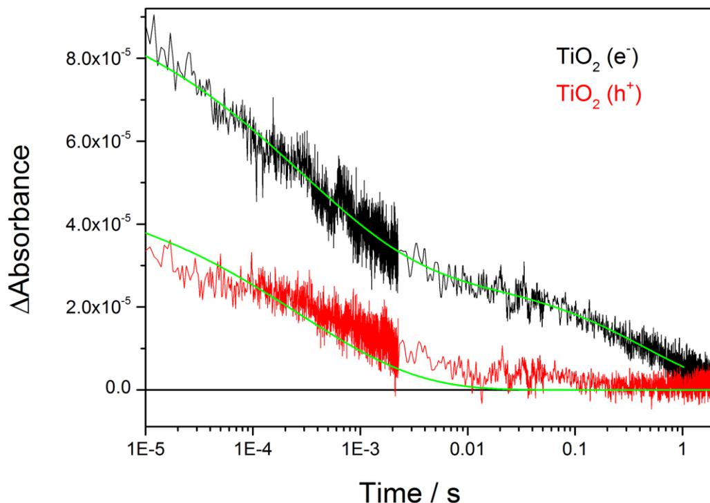
**Figure S5:** TA decay traces of *nc*-TiO<sub>2</sub> holes and photoelectrons recorded 460 nm and 900 nm respectively following the UV excitation (355 nm, 35 μJ cm<sup>-2</sup>, SE) of *nc*-TiO<sub>2</sub> (1.1 μm) in 0.5M NaClO<sub>4(aq)</sub> (pH 2) at 0 V vs Ag/AgCl. The same fast component present in both traces is assigned to electron-hole recombination.
