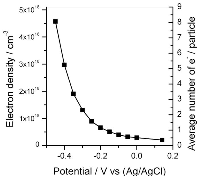
**Figure S3.** Change in electron density measured by charge extraction stepping from the value indicated to +0.44V (vs. Ag/AgCl) in the dark, 0.5 M NaClO<sub>4</sub> (pH 2), nc-TiO<sub>2</sub> electrode (4 μm).
