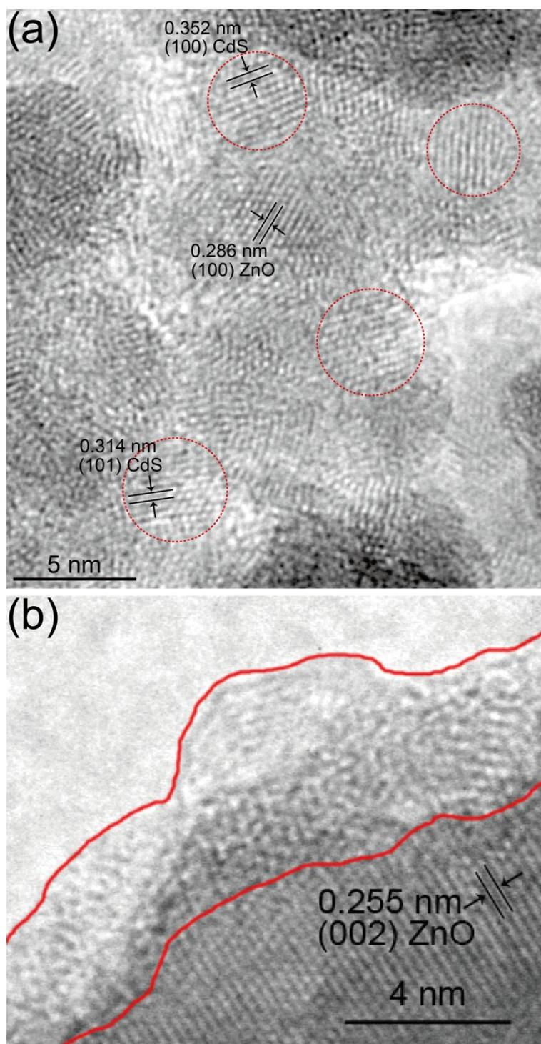
**Fig. S2** HRTEM images of CdS QDs on ZnO film recorded using a JEM-2010 TEM from JEOL Ltd.. (a) shows that a hexagonal CdS is deposited on ZnO by the SILAR method and its crystal size is about 3.5 nm (marked out by red circles). (b) shows that the thickness of the CdS shell coated on ZnO is about 3-5 nm (marked out by red lines).
