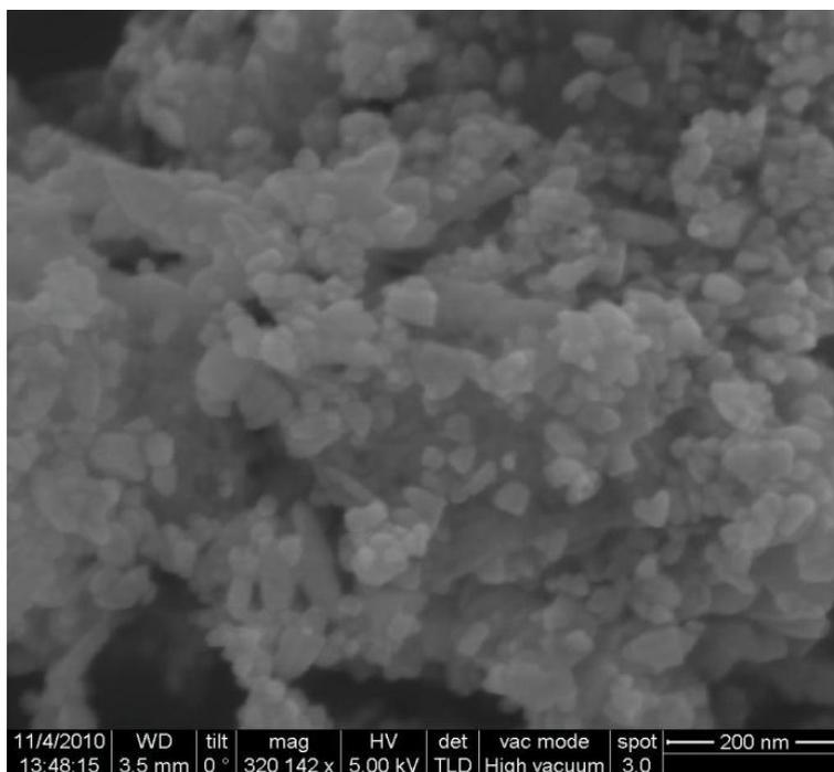
**Fig. S1** SEM image of the as-synthesized ZnO nanoparticles in a continuous flow supercritical reactor recorded using a Nova 600 Nano SEM from FEI. The size of ZnO particle is about 20 nm.
