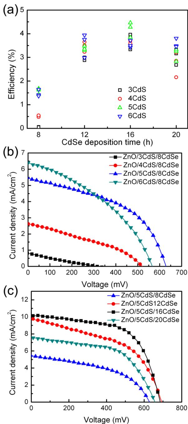
**Fig. S3** (a) Efficiencies of the tested QDSCs. The typical  $J$ - $V$  curves for QDSCs fabricated with (b) different CdS SILAR cycles and the same CdSe CBD deposition time (8 h), (c) the same CdS SILAR cycle (5 cycles) and different CdSe CBD deposition time.
