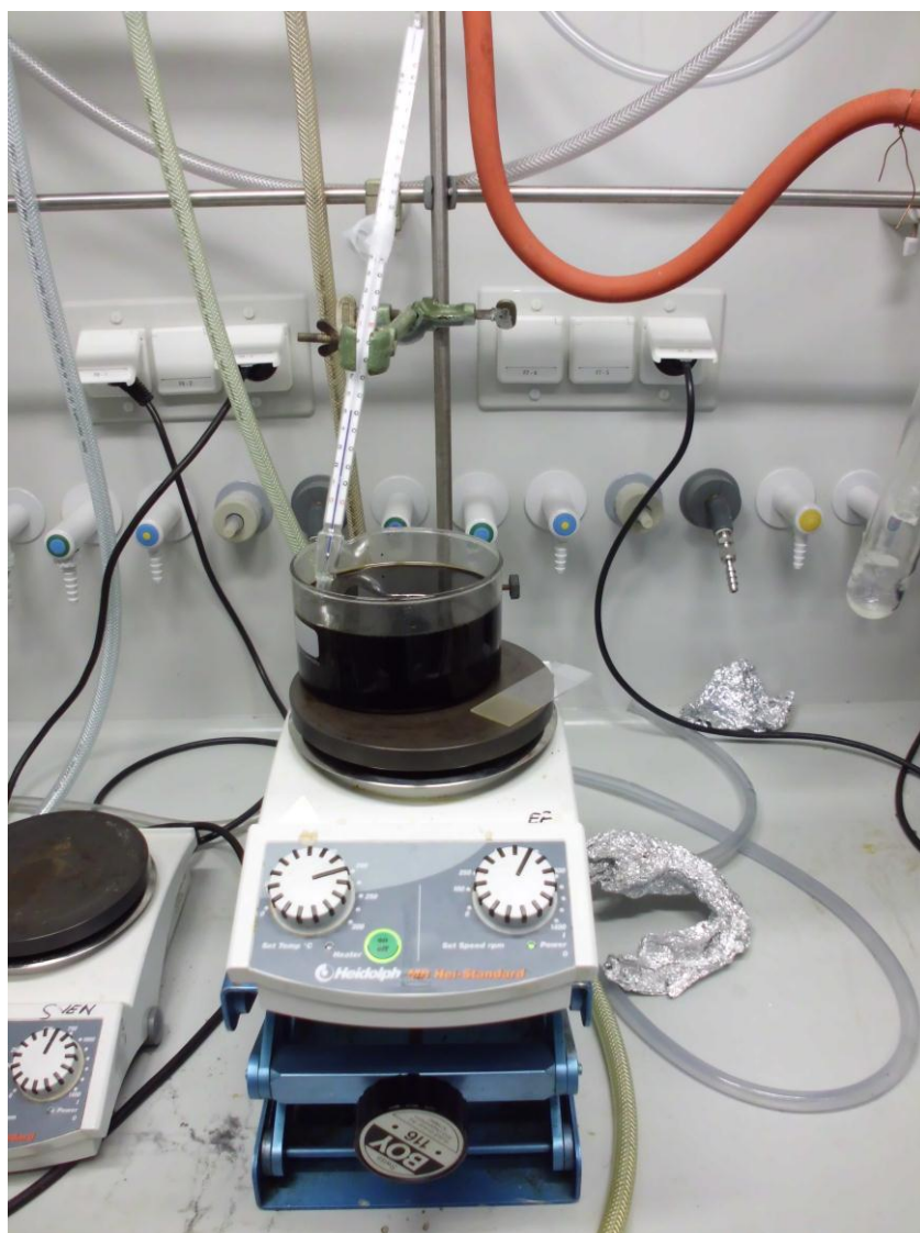
SI Figure 3. Heating of the dip-coated film to observe the color change.
