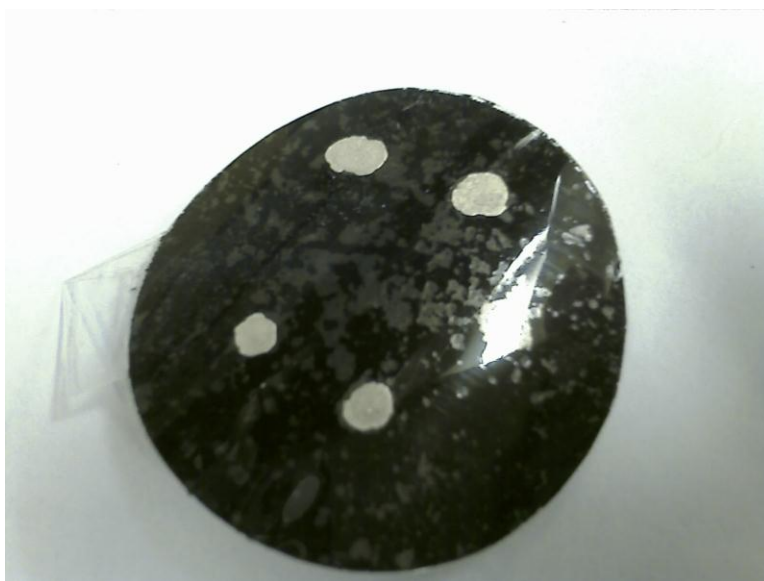
Fig. S2. Photograph of the underside of the Buckypaper-on-tape showing the silver contacts aligned with the adhesive tape.
