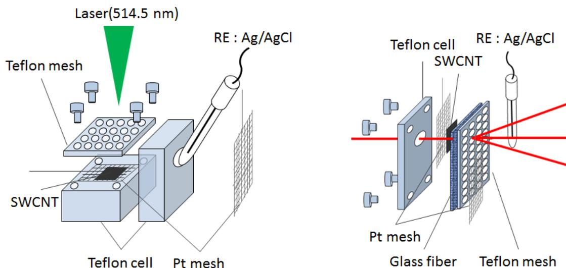
**Fig. S1** In situ cell for Raman scattering study(a), X-ray diffraction(b).
