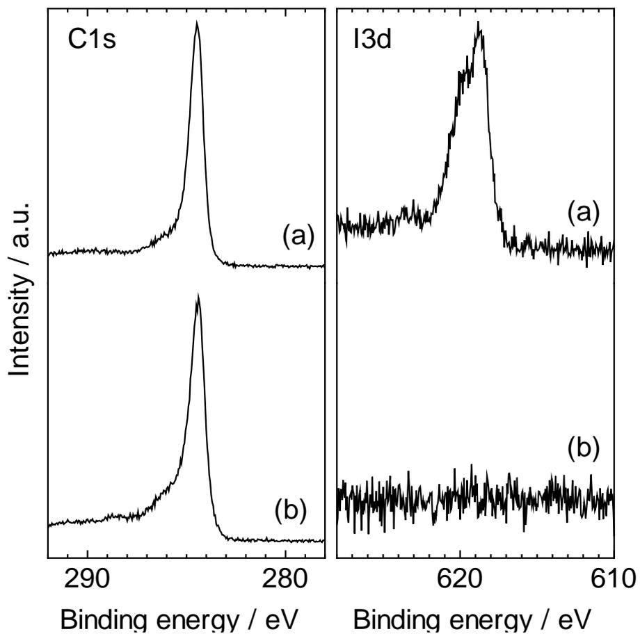
**Fig. S2** XPS spectra of iodine doped SWCNT(a), and pristine SWCNT(b).
