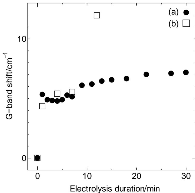
**Fig. S5** G-band shift related to electrolysis duration observed by in-situ Raman study. Electrolytes used were neutral (a) and acidic (in HI) (b) aqueous NaI solutions.
