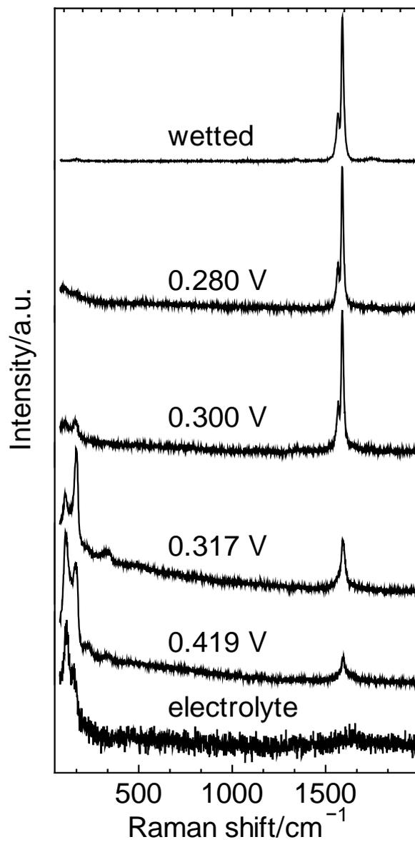
**Fig. S4** In-situ Raman spectra at the various applied potential.
