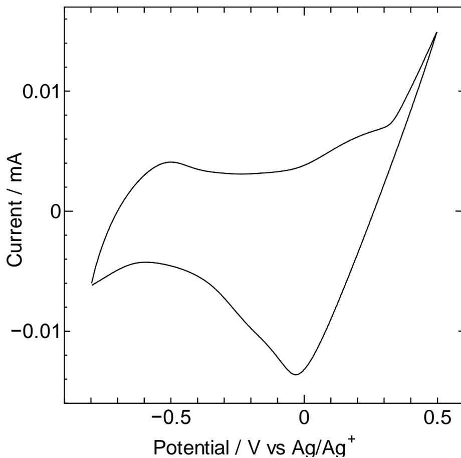
**Fig. S3** Cyclic voltammetry of SWCNT in 1 M NaI aqueous solution. Working electrode : SWCNT, counter electrode : Pt mesh/activated carbon fiber, and reference electrode : Ag/Ag<sup>+</sup> are fabricated. The scan rate was 100 mV/s.
