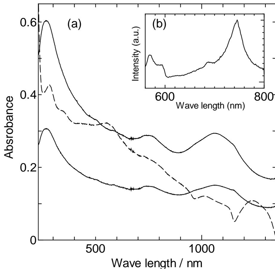
**Fig. S6** UV-VIS absorbance of 10  $\mu\text{g/mL}$ (top), 5  $\mu\text{g/mL}$ (bottom) SWCNT:SDS aqueous solution(solid) and iodine doped SWCNT(dash) (a), photo luminescence spectrum of iodine doped SWCNT excited by 514.5 nm(b).
