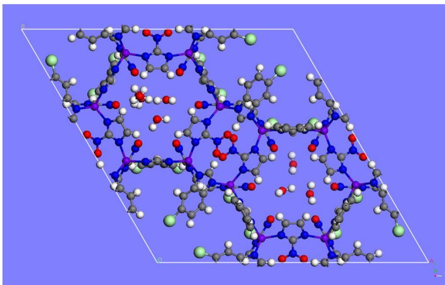
**Fig. S18** Simulated pure water adsorption snapshot in ZIF-69 (298K, 0.2 bar). (Grey = Carbon, red = Oxygen, white = Hydrogen, blue = Nitrogen, purple = Zinc, teal = Chlorine)
