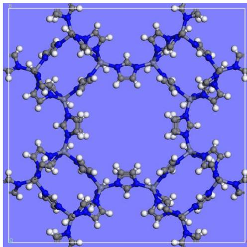
**Fig. S1** ZIF-10 unit cell. ZIF-10 belongs to the MER topology. In the ZIF-10 framework, each Zn atom is bridged by four imidazolate (IM) linkers. The unit cell lengths of ZIF-10 are:  $a = 27.061 \text{ \AA}$ ,  $b = 27.061 \text{ \AA}$ ,  $c = 19.406 \text{ \AA}$ , and angles  $\alpha = 90^\circ$ ,  $\beta = 90^\circ$ ,  $\gamma = 90^\circ$ .
