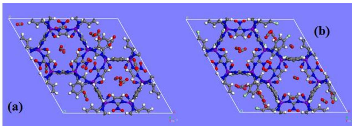
**Fig. S12** Simulated pure CO<sub>2</sub> adsorption snapshot in ZIF-68 (298K, 0.3bar). (Grey = Carbon, red = Oxygen, white = Hydrogen, blue = Nitrogen, purple = Zinc)
