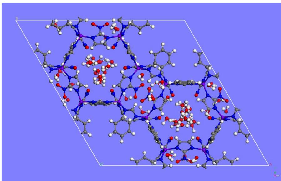
**Fig. S16** Simulated pure water adsorption snapshot in ZIF-68 (298K, 0.2 bar). (Grey = Carbon, red = Oxygen, white = Hydrogen, blue = Nitrogen, purple = Zinc)
