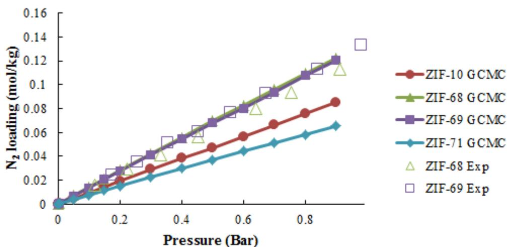
**Fig. S10** Simulated pure N<sub>2</sub> isotherms in ZIF-10, ZIF-68, ZIF-69 and ZIF-71 up to 1 bar pressure at 298K.
