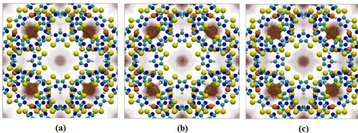
**Fig. S14** Simulated adsorption density profiles in ZIF-71 (a) CO<sub>2</sub> adsorbed from a CO<sub>2</sub>/N<sub>2</sub> (15%/85%) mixture, (b) SO<sub>2</sub> and (c) CO<sub>2</sub> adsorbed from a CO<sub>2</sub>/N<sub>2</sub>/SO<sub>2</sub> (15%/81%/4%) mixture, (cyan = carbon, white = hydrogen, red = oxygen, orange = zinc, yellow = chlorine).
