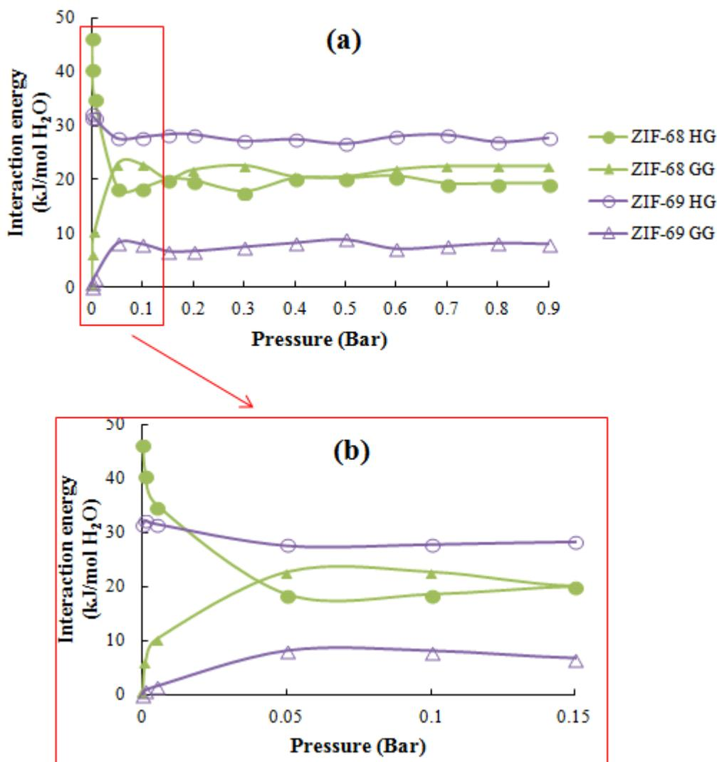
**Fig. S19** Host-guest (HG) and guest-guest (GG) interaction energies for water adsorption in ZIF-68 and ZIF-69 at 298K as a function of H<sub>2</sub>O pressure.
