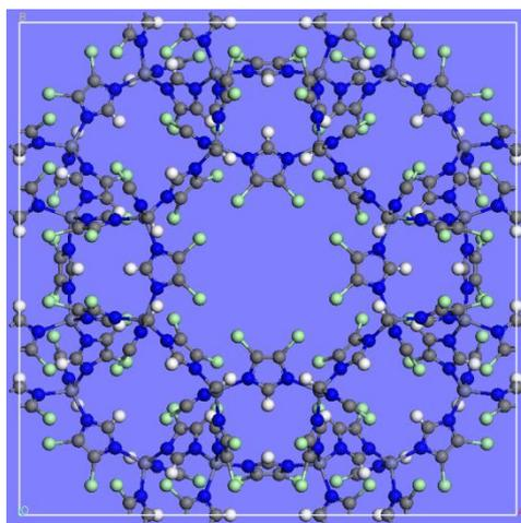
**Fig. S4** ZIF-71 unit cell. ZIF-71 has the RHO topology. In the ZIF-71 framework, each Zn atom is bridged by 4,5-dichloroimidazolate (dcIM). The framework contains large cages of connected by small windows. The unit cell lengths of ZIF-71 are:  $a = 28.554 \text{ \AA}$   $b = 28.554 \text{ \AA}$ ,  $c = 28.554 \text{ \AA}$ , and angles  $\alpha = 90^\circ$ ,  $\beta = 90^\circ$ ,  $\gamma = 90^\circ$ .
