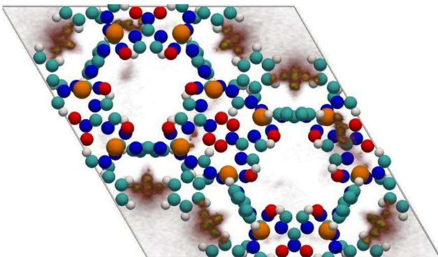
**Fig. S17** Simulated CO<sub>2</sub> adsorption density profile from a CO<sub>2</sub>/N<sub>2</sub>/SO<sub>2</sub>/H<sub>2</sub>O (15%/80.9%/0.1%/4%) mixture in ZIF-68. (cyan = carbon, white = hydrogen, red = oxygen, yellow = chlorine, orange = zinc).
