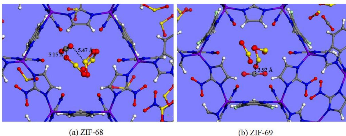
**Fig. S15** Simulated adsorption snapshots (a) in ZIF-68, (b) in ZIF-69 from CO<sub>2</sub>/N<sub>2</sub>/SO<sub>2</sub> (15%/81%/4%) mixture 298K 1 bar. (Grey = Carbon, red = Oxygen, white = Hydrogen, blue = Nitrogen, purple = Zinc, Teal = Chlorine)
