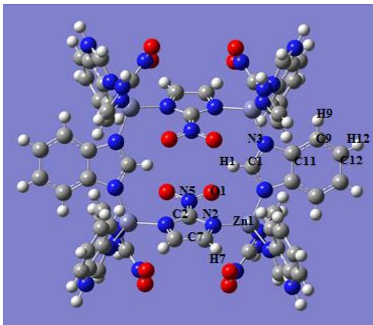
**Fig. S6** Cluster  $(\text{Zn}_4\text{C}_{60}\text{N}_{30}\text{H}_{50}\text{O}_{12})^{+4}$  used for deriving partial charges on ZIF-68
