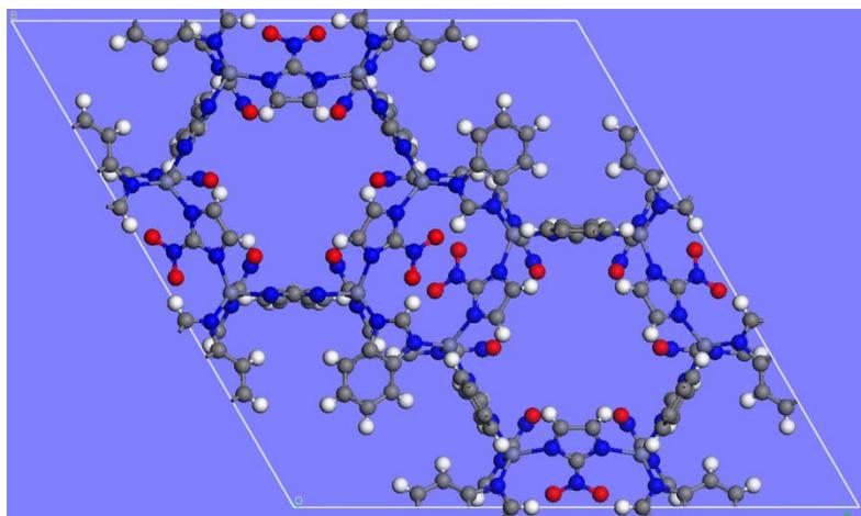
**Fig. S2** ZIF-68 unit cell. ZIF-68 has the GME topology. In the ZIF-68 framework, each Zn atom is bridged by two different linkers: benzimidazole (bIM) and 2-nitroimidazole (nIM). The framework has small side pockets as well as large pore channels. The unit cell lengths of ZIF-68 are:  $a = 26.64 \text{ \AA}$ ,  $b = 26.64 \text{ \AA}$ ,  $c = 18.488 \text{ \AA}$ , and angles  $\alpha = 90^\circ$ ,  $\beta = 90^\circ$ ,  $\gamma = 120^\circ$ .
