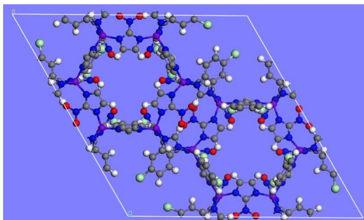
**Fig. S3** ZIF-69 unit cell. ZIF-69 has the GME topology. In the ZIF-68 framework, each Zn atom is bridged by two different linkers: 5-chlorobenzimidazole (cbIM) and 2-nitroimidazole (nIM). The framework has small side pockets as well as large pore channels. The unit cell lengths of ZIF-69 are:  $a = 26.084 \text{ \AA}$   $b = 26.084 \text{ \AA}$ ,  $c = 19.408 \text{ \AA}$ , and angles  $\alpha = 90^\circ$ ,  $\beta = 90^\circ$ ,  $\gamma = 120^\circ$ .
