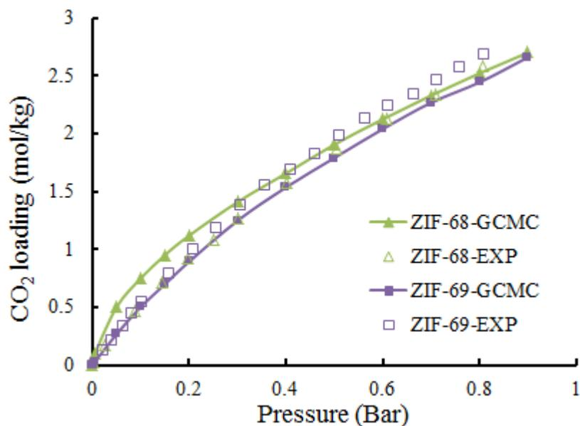
**Fig. S9** Comparison of simulated pure CO<sub>2</sub> isotherms and experimental data<sup>5</sup> in ZIF-68 and ZIF-69 up to 1 bar pressure at 273K. (GCMC = simulated data, EXP = experimental data)
