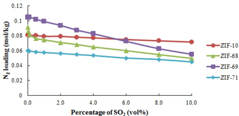
**Fig. S11** The N<sub>2</sub> uptake as a function of SO<sub>2</sub> feed concentration from flue gas mixture in ZIF-10, ZIF-68, ZIF-69 and ZIF-71 up to 1 bar pressure.
