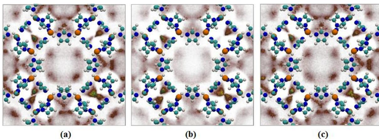
**Fig. S13** Simulated adsorption density profiles in ZIF-10 (a) CO<sub>2</sub> adsorbed from a CO<sub>2</sub>/N<sub>2</sub> (15%/85%) mixture, (b) SO<sub>2</sub> and (c) CO<sub>2</sub> adsorbed from a CO<sub>2</sub>/N<sub>2</sub>/SO<sub>2</sub> (15%/81%/4%) mixture, (cyan = carbon, white = hydrogen, red = oxygen, orange = zinc).
