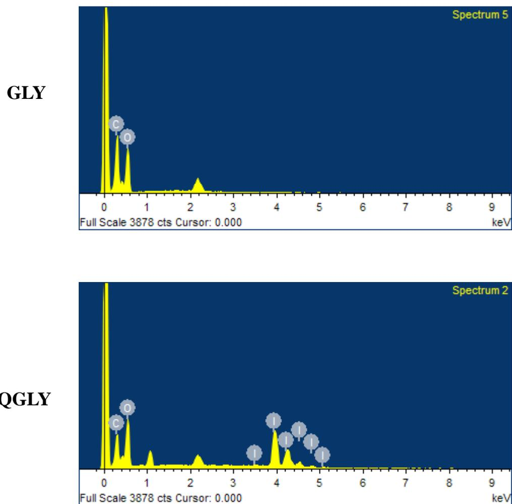
**Fig. S3.** EDS spectra of GLY and QGLY.
