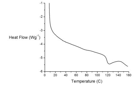
**Figure S4.** Differential scanning calorimetry of poly(methyl methacrylate). The glass transition temperature ( $T_g$ ) was determined to be below 140 °C (temperature used to bake films to ensure that they were melted for "erasing" steps).
