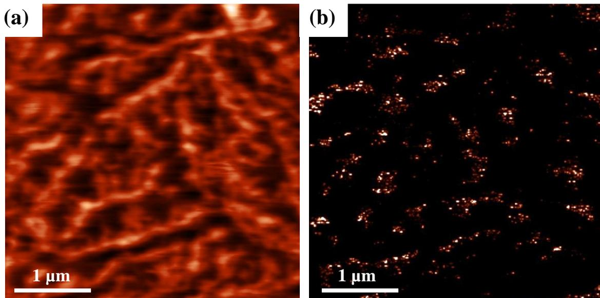
**Figure S3.** (a) The morphology and (b) the corresponded current map (tip bias=0.3V) of the FW PND network
