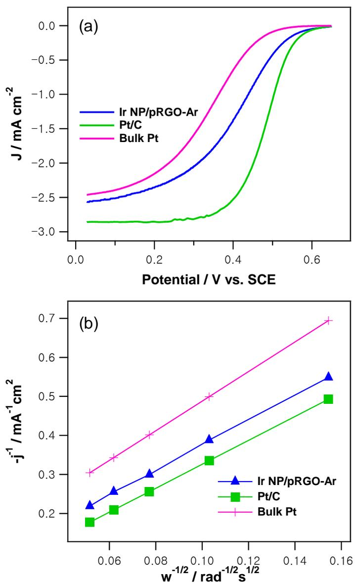
**Fig. S4.** Comparison of (a) RDE voltammograms and (b) K-L plots (at +0.1 V vs. SCE) for ORR in an  $\text{O}_2$ -saturated 0.5 M  $\text{H}_2\text{SO}_4$  solution at GC electrodes modified with Ir NP/pRGO-Ar, commercial Pt/C, and bulk Pt (disk electrode, Pt disk diameter = 3 mm). Rotation speed, 900 rpm and scan rate, 10  $\text{mV s}^{-1}$ . Current densities ( $J$ ) were obtained via the current normalization with respect to the corresponding electrode GSA, as determined by the CC method.
