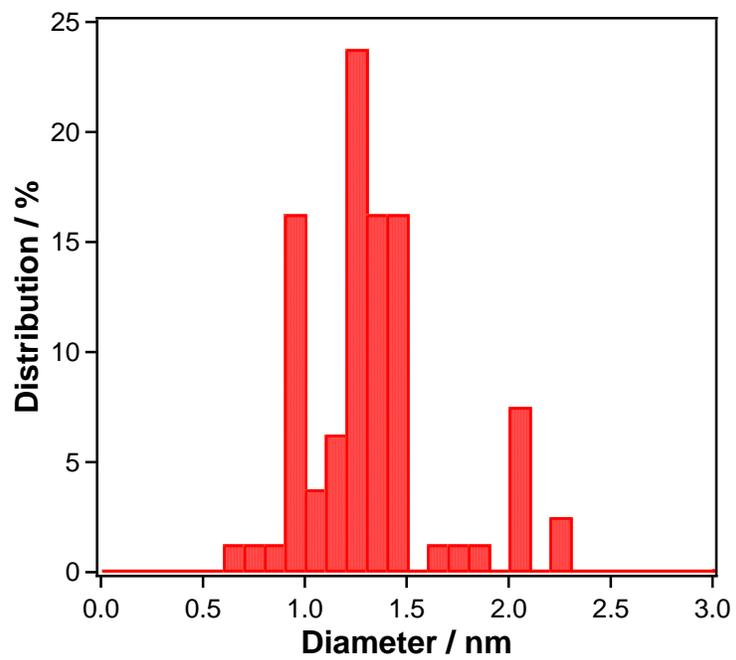
**Fig. S2.** Particle size distribution of the Ir nanoparticles immobilized on pRGO nanosheets.
