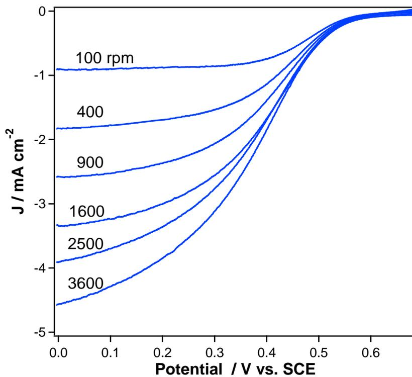
**Fig. S5.** RDE voltammograms for ORR in an  $\text{O}_2$ -saturated 0.5 M  $\text{H}_2\text{SO}_4$  solution at the Ir NP/pRGO-Ar-modified GC electrode depending on rotation speed with a scan rate of  $10 \text{ mV s}^{-1}$ .
