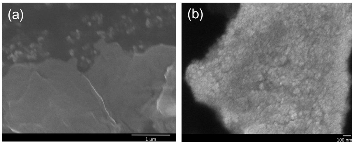
**Fig. S1.** Typical SEM images of (a) pRGO and (b) Ir NP/pRGO nanocomposites.
