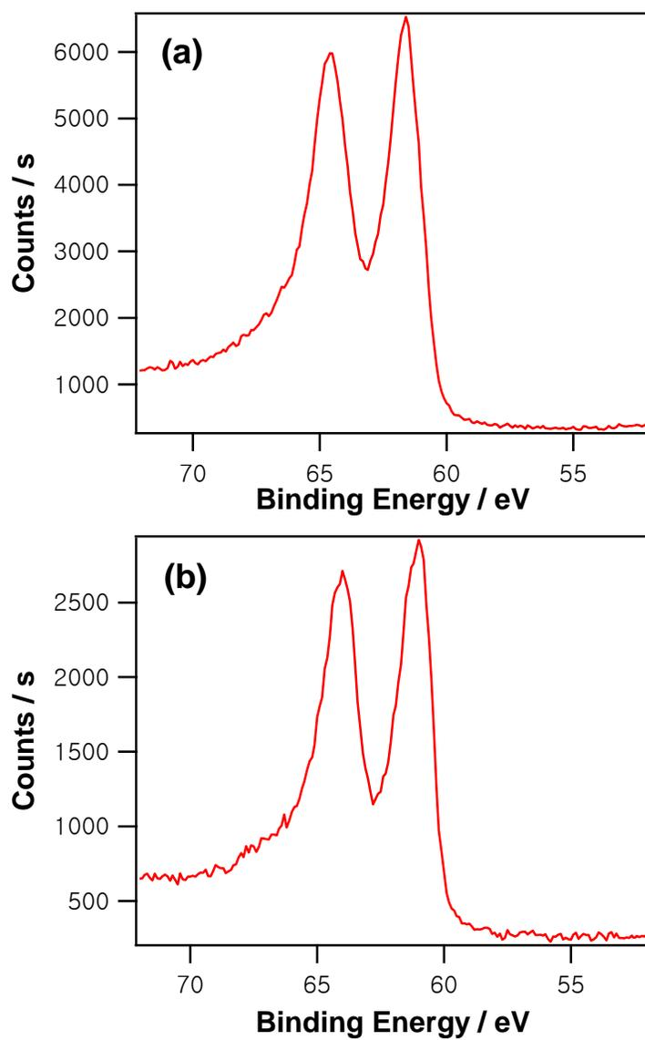
**Fig. S3.** XPS spectra of (a) Ir NP/pRGO-air and (b) Ir NP/pRGO-H<sub>2</sub> for Ir 4f region.
