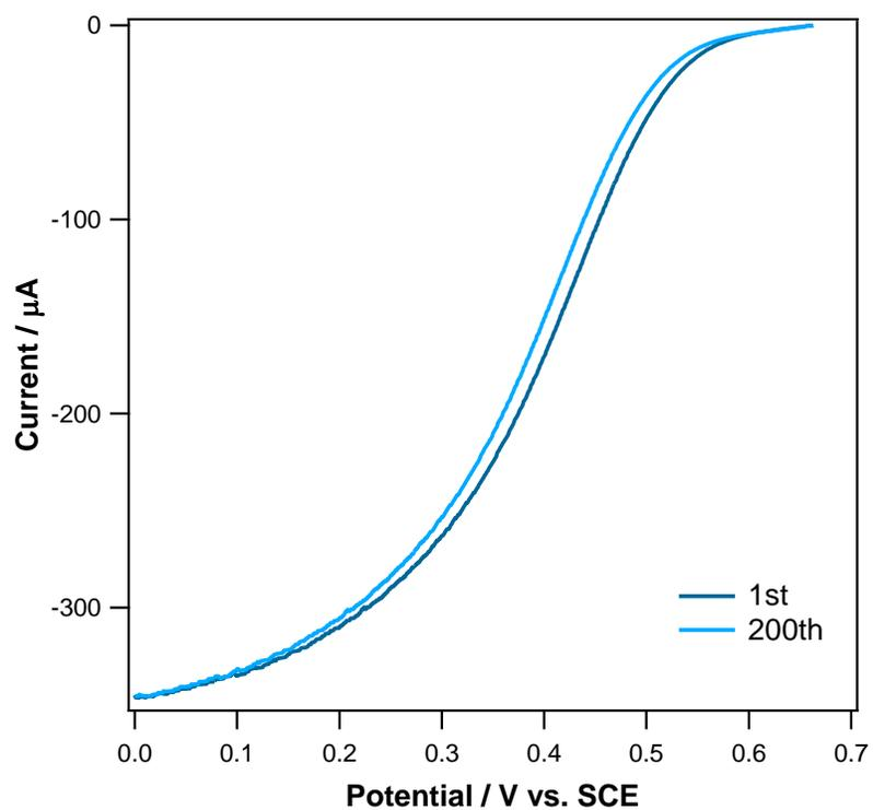
**Fig. S6.** RDE voltammograms before and after repetitive 200 runs obtained with Ir NP/pRGO-Ar-modified GC electrode in an  $\text{O}_2$ -saturated 0.5 M  $\text{H}_2\text{SO}_4$  solution at a rotation rate of 1600 rpm. All the other conditions are the same as in Figure 5.
