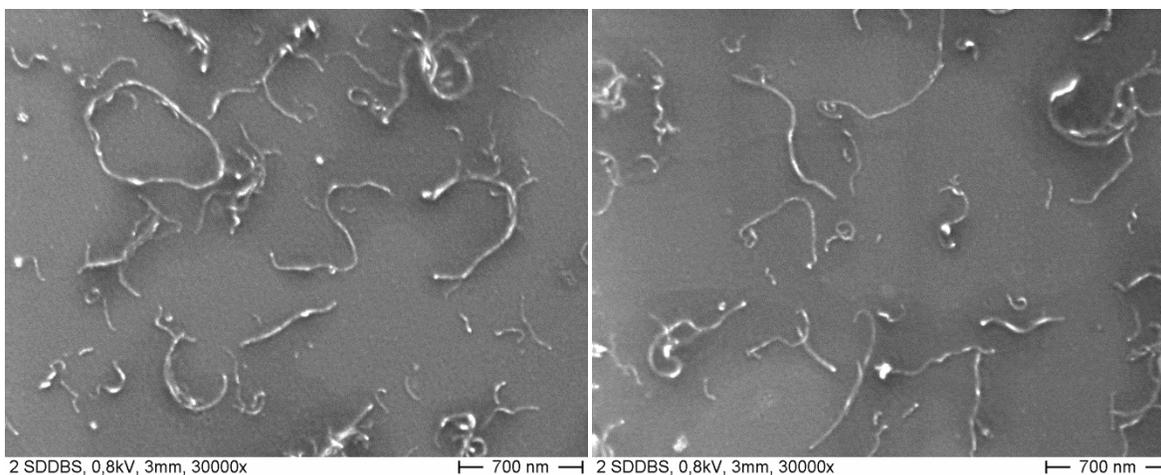
**Figure 3S** SEM images of dispersed MWCNTs in 1 wt% SDDBS.
