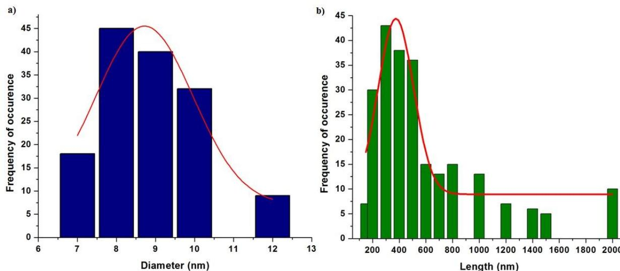
**Figure 4S** Diameter and length distributions of the dispersed MWCNTs with SDDBS
