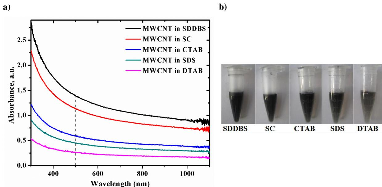
**Figure 1S.** (a) UV-vis spectra of CNTs in SDDBS (black), SC (red), CTAB (blue), SDS (green) and DTAB (pink). (b) Photograph of their supernatants after centrifuge.
