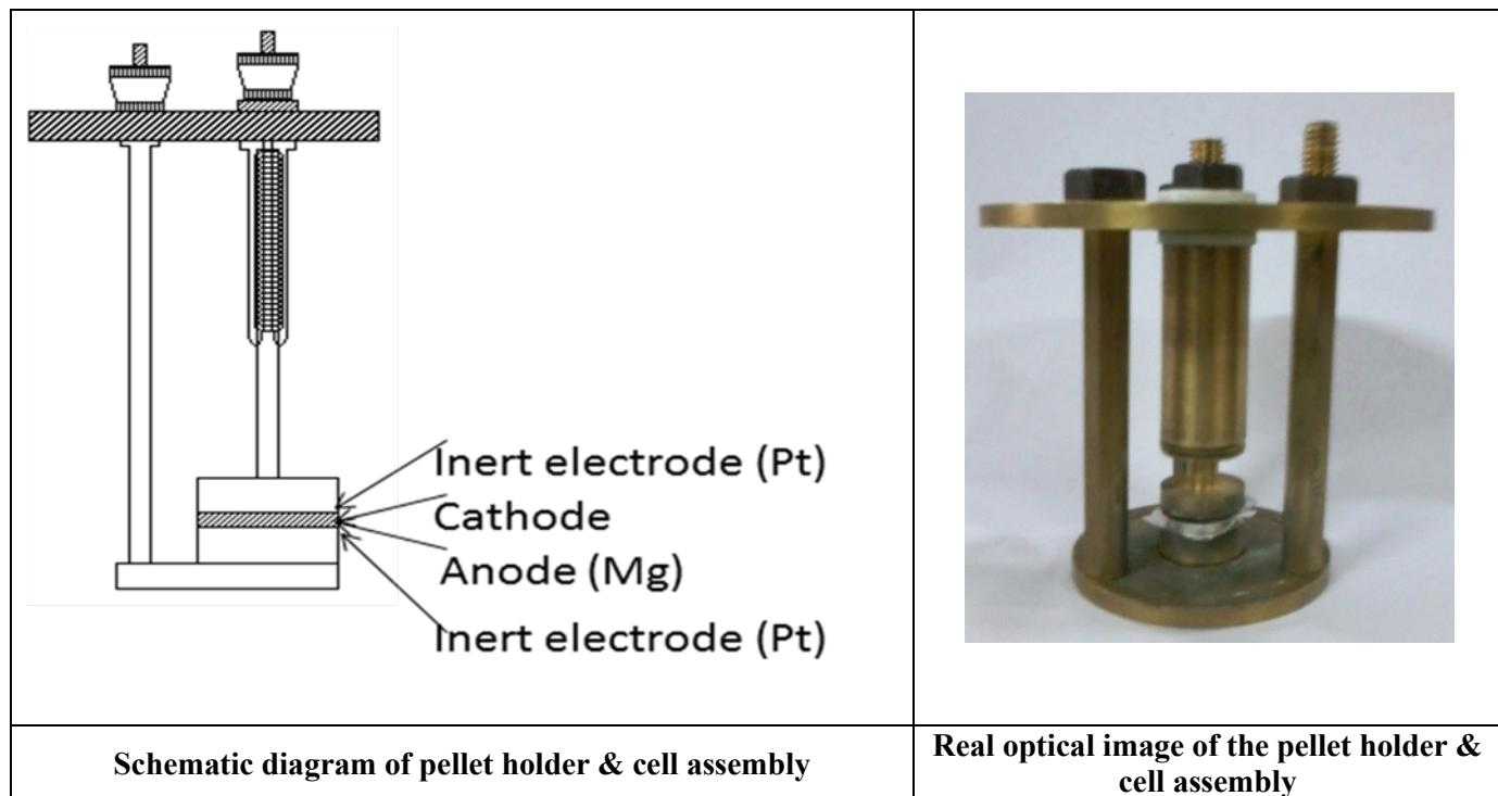
**Figure S-5:** Schematic diagram and real photograph of spring loaded brass pellet holder used for assembling cell.
