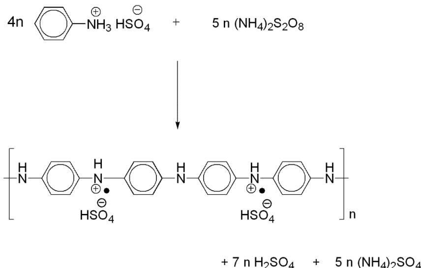
**Figure S-3:** Polymerization reaction of protonated aniline monomer.
