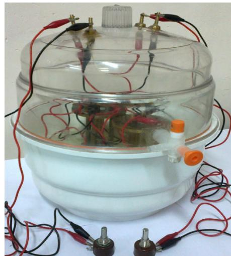
**Figure S-6:** Cell assembled in a spring loaded brass pellet holder secured in moisture free desiccators under ambient conditions.
