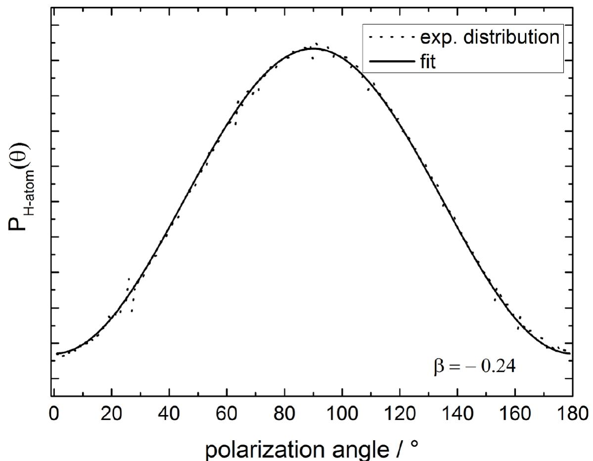
Angular distribution of H-atom photofragments produced in the photodissociation of phthalide. The experimental distribution was fitted with expression (2) as given in the main paper. As visible the distribution is anisotropic and a  $\beta$ -parameter of -0.24 is obtained.
