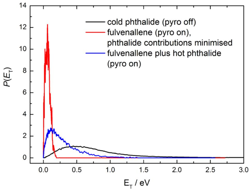
The figure presents a comparison of H-atom translational energy distributions. The black line corresponds to H-atoms from cold phthalide (similar to figure a). The red line represents the distribution from fulvenallene, selected from the image with pyrolysis on around  $0^\circ$  as depicted in figure 6. The blue line finally represents a selected part of the image with pyrolysis on around  $90^\circ$ . It contains both contributions, *i.e.* is perturbations from hot phthalide are present.
