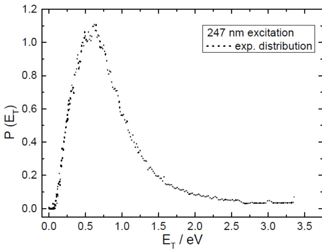
Translational energy distribution of H-atoms produced in the photodissociation of phthalide. The distribution peaks at 0.58 eV, while the distribution of H-atoms from fulvenallene peaks at 0.05 eV. Electrons with a kinetic energy release of up to 3 eV are formed. Overall the distribution differs significantly from the one derived for  $\text{C}_7\text{H}_6$ . Note that the H-atoms originate from a two-photon excitation of phthalide.
