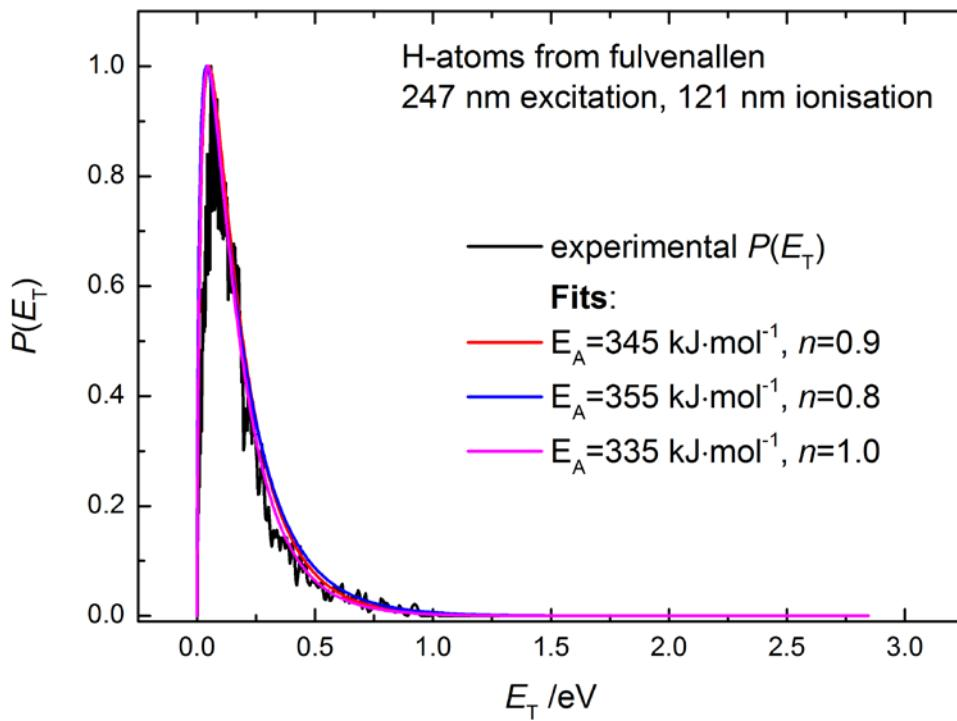
The translational energy distribution of H-atoms from fulvenallene is described by expression (1). Here the dependence of the fitting parameter  $n$  in expression (1) on the activation barrier/excess energy is shown. As visible a change of the activation barrier by  $\pm 10 \text{ kJ}\cdot\text{mol}^{-1}$  does not change  $n$  significantly.
