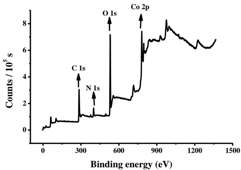
Figure S7. The XPS survey data of CoO<sub>x</sub>-4 electrodeposited at +1.5 V in borate buffer at pH 9.2.
