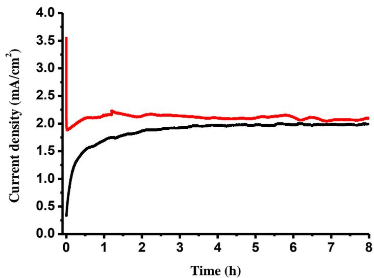
**Figure S2.** Current density profiles of electrodeposition at +1.1 V containing 1.0 mM cobaloxime **1** (black plot) and current density profiles of the as-synthesized CoOx-**1** for bulk electrolysis at +1.1 V in a cobaloxime-free solution (red plot).
