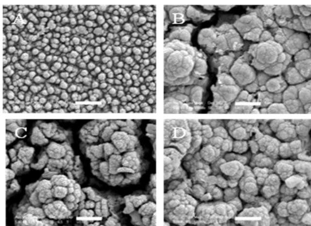
Figure S3. SEM micrographs of catalysts deposited on FTO surface after 7 h of electrolysis at +1.5 V vs Ag/AgCl with 1 mM cobaloximes in a 0.1 M borate buffered solution at pH 9.2. The initial cobaloximes are: (A) 1, (B) 2, (C) 3, (D) 4. Scale bar: 1  $\mu\text{m}$ .
