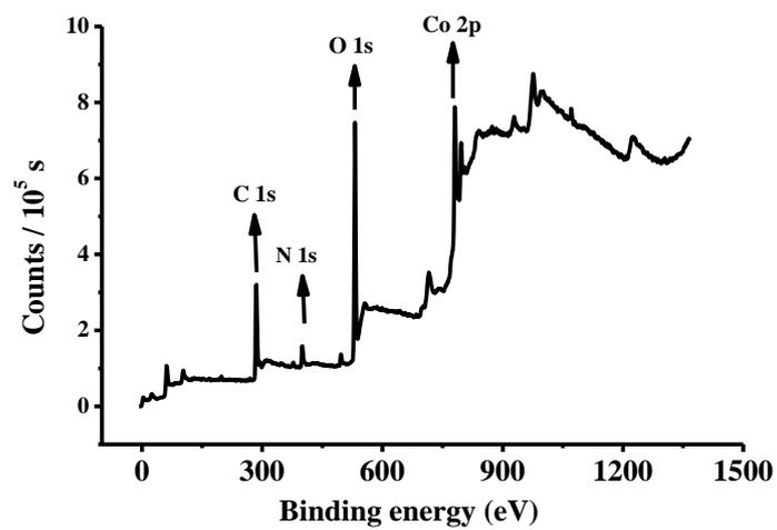
Figure S6. The XPS survey data of CoO<sub>x</sub>-3 electrodeposited at +1.5 V in borate buffer at pH 9.2.
