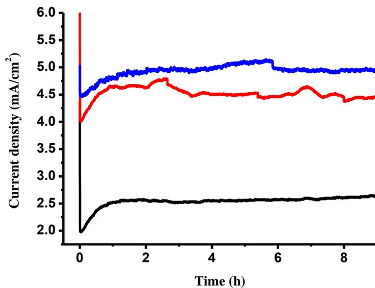
**Figure S1.** Current density profile of CoO<sub>x</sub>-1 catalyst (deposited at +1.5 V) for bulk electrolyses at 1.1V in a cobaloxime-free solution: 0.1 M KBi (black plot), 0.3 M KBi (red plot), 0.5 M KBi (blue plot).
