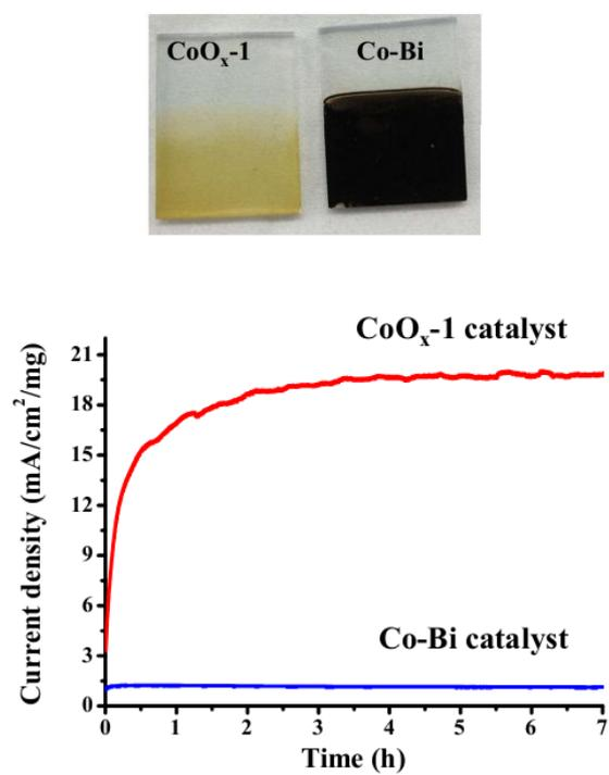
Figure S4. Current density profiles by weight of CoO<sub>x</sub>-1 (red plot) and Co-Bi (blue plot) catalyst electrodeposited under the same conditions in borate buffer at pH 9.2.
