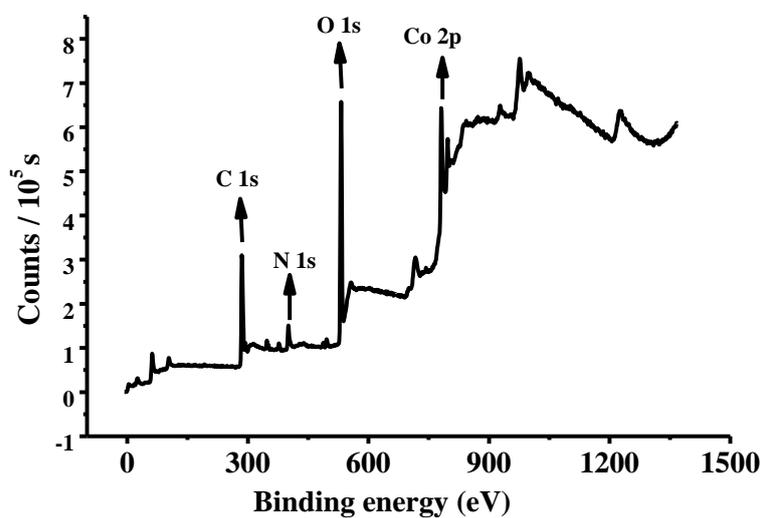
Figure S5. The XPS survey data of  $\text{CoO}_x$ -2 electrodeposited at +1.5 V in borate buffer at pH 9.2.
